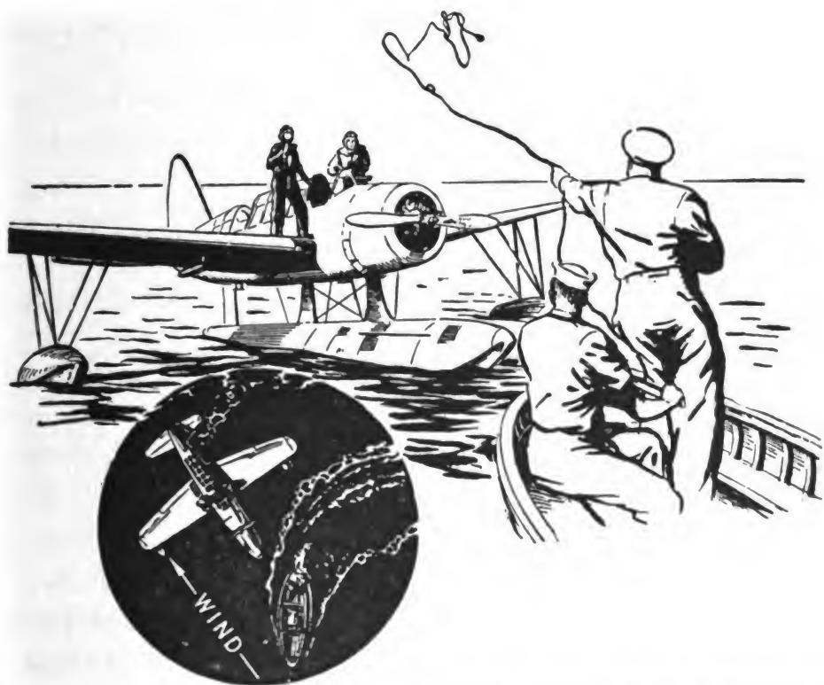
Figure 37.—Small boat approaching a seaplane. Inset—Method of approaching a drifting seaplane.
