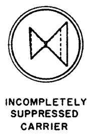
Figure 105. Double-trapezoid patterns observed on phase-shift ssb transmitter.
