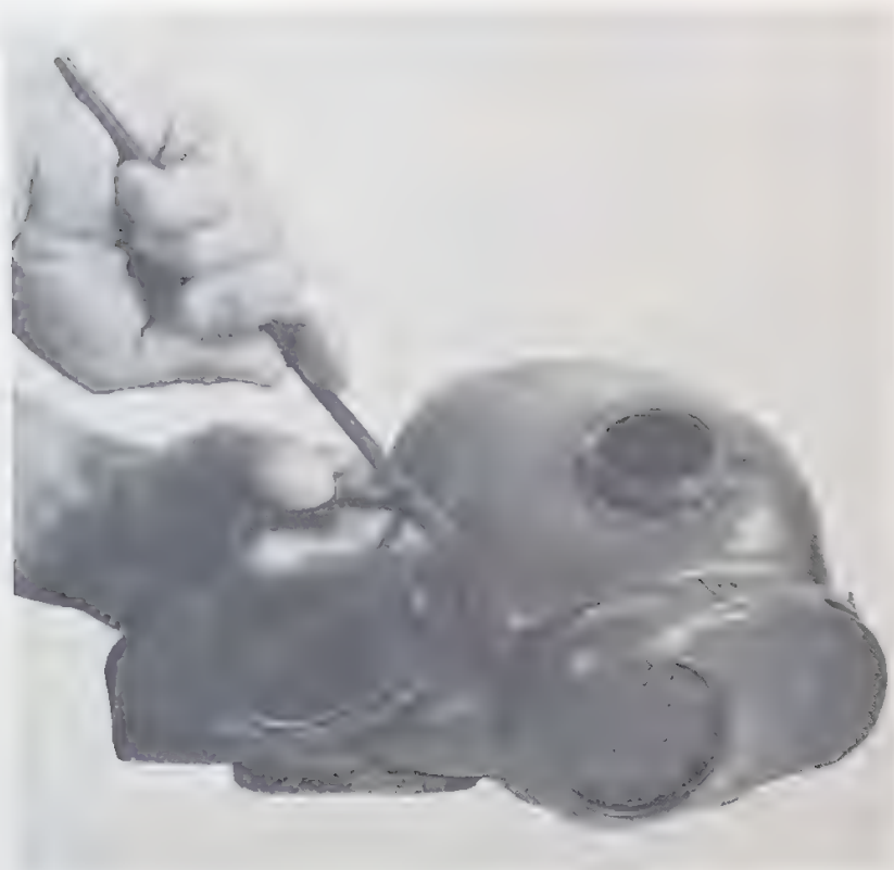
Figure 18. Bending tabs of eyering with eyering hook tool.
