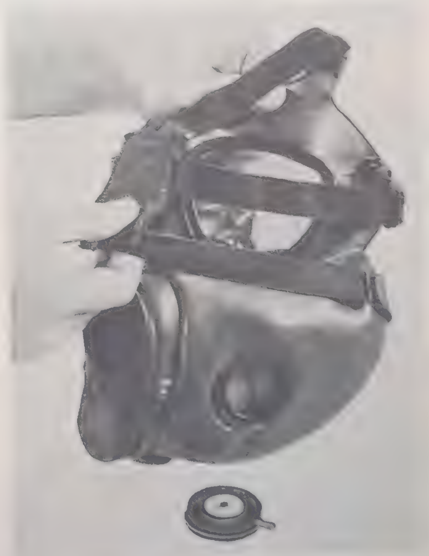
Figure 13. Reversing the head harness.
