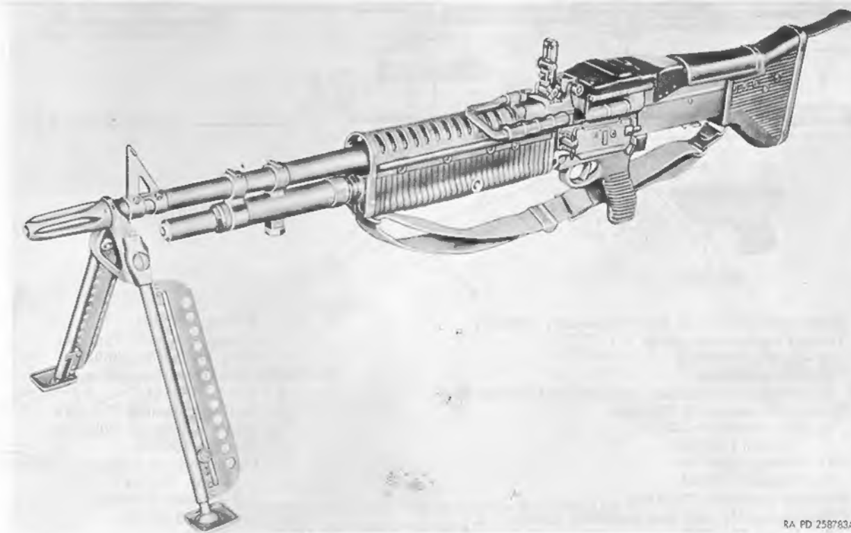
Figure 3. 7.62-mm machinegun M60 - left front view.
