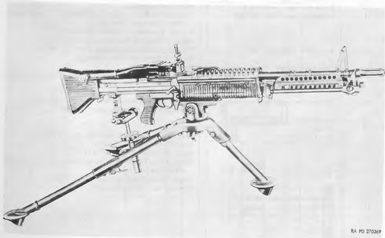
Figure 2. 7.62-mm machinegun M60 on machinegun tripod mount M122 - right side view.
