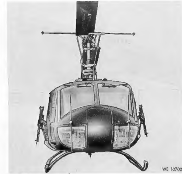
Figure 1-1. 7.62-millimeter machine gun helicopter armament subsystem XM23—installed on UH-1D helicopter.
