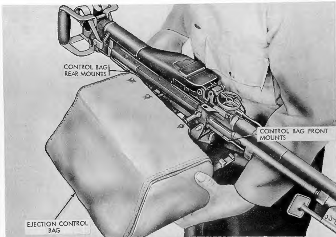
STEP 1 - POSITION EJECTION CONTROL BAG UNDER BAG MOUNTS.
