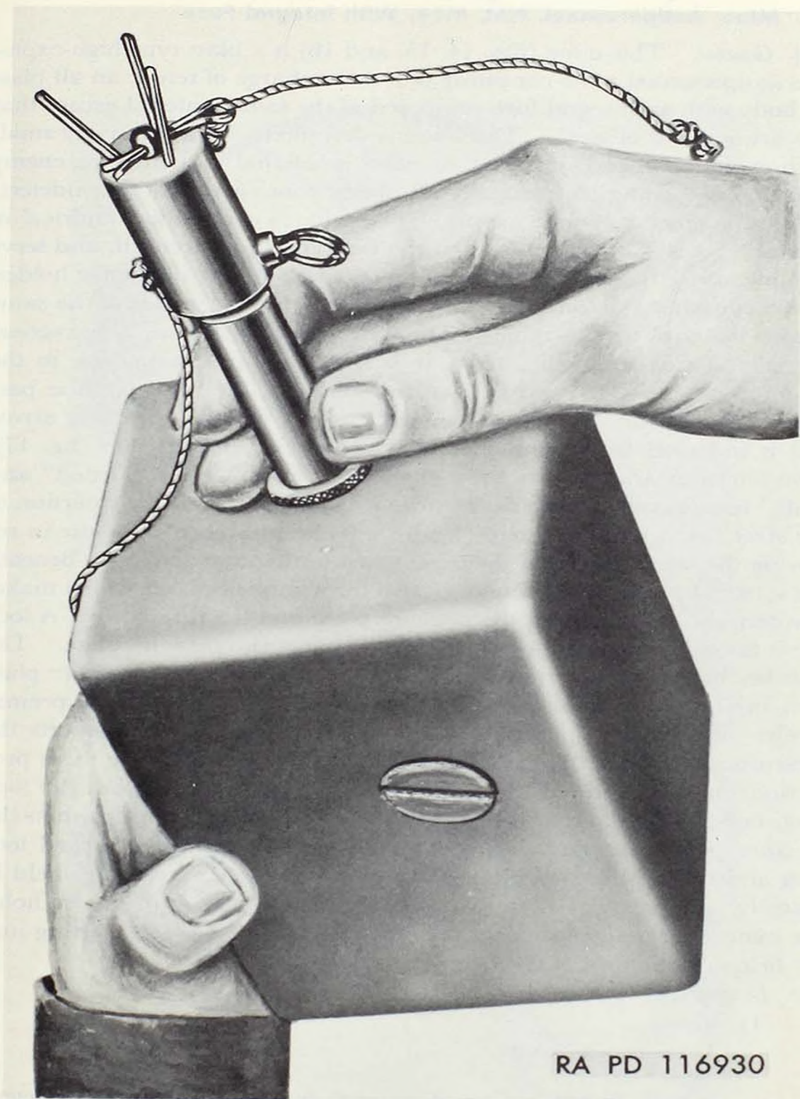
Figure 13. Installing fuze M7A1 in antipersonnel mine M3.
