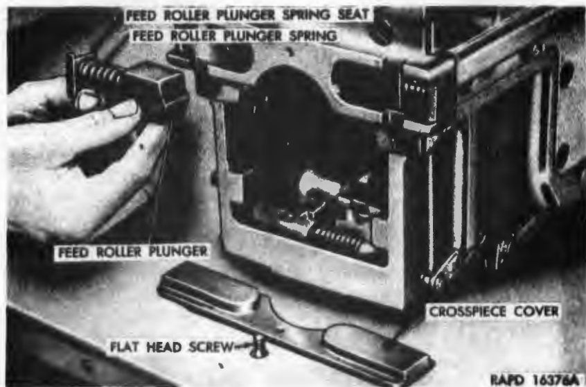
Figure 333. Replacing feed roller plunger springs.
