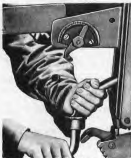
SHELL PUSHER WITH FLAT END INSERTED BETWEEN FEED ROLLERS FORCING ROUNDS UPWARD INTO CARTRIDGE REMOVER
