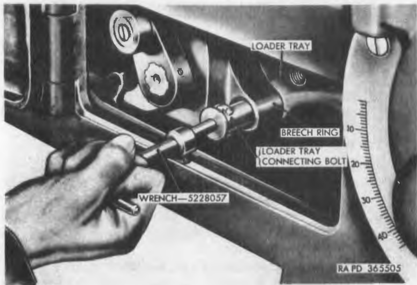
Figure 325. Removing loader tray connecting bolt.
