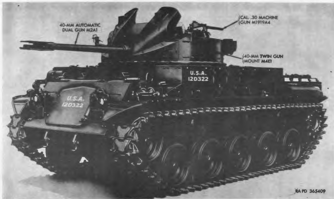
Figure 1. Twin 40-mm full tracked self-propelled gun M42 (T141), with guns in firing position—left front view.
