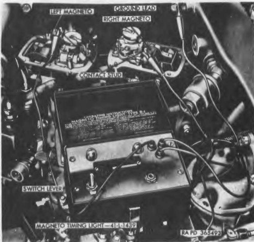
Figure 117. Synchronizing magnetos on engine with magneto timing light 41-L-1439.
