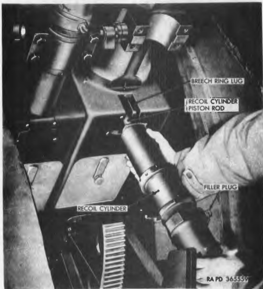
Figure 290. Removing or installing recoil cylinder.
