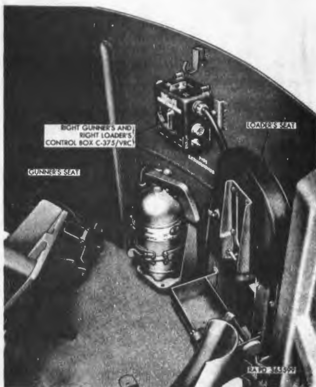
Figure 371. Right gunner's and loader's control box C-375/VRC.
