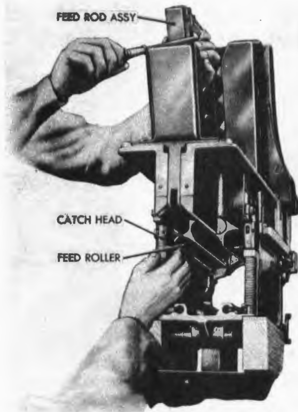
Figure 330. Removing feed rod assembly.
