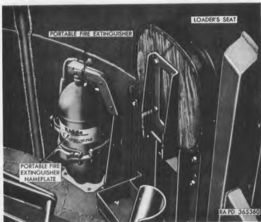
Figure 63. Portable fire extinguisher.
