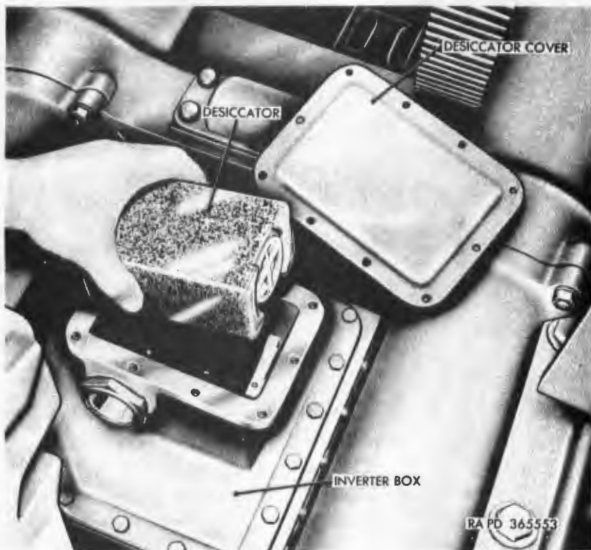
Figuree 271. Replacing desiccator in inverter box.
