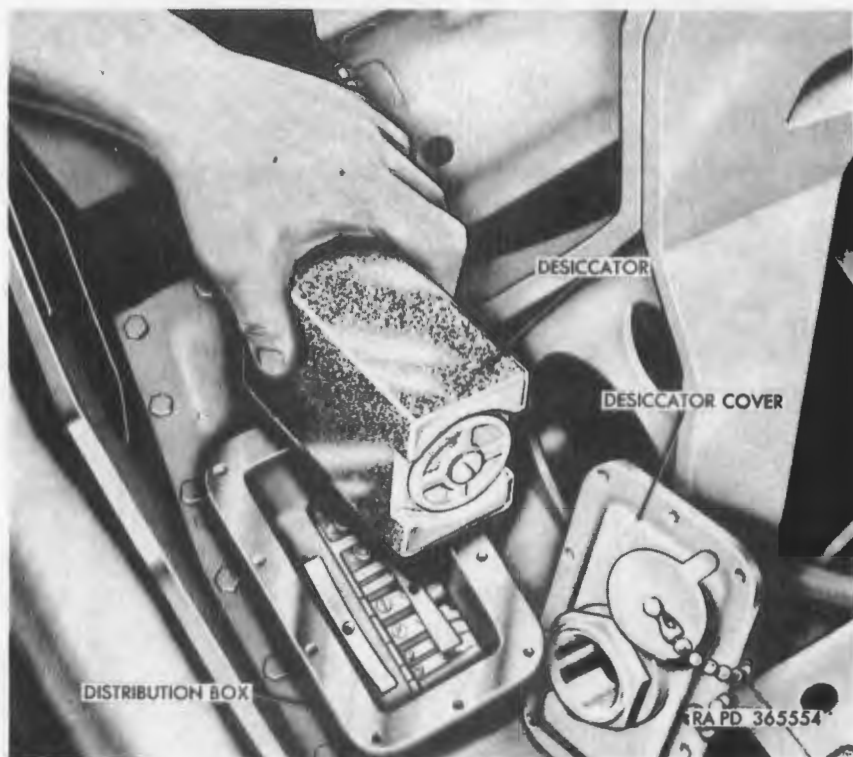
Figure 272. Replacing desiccator in distribution box.
