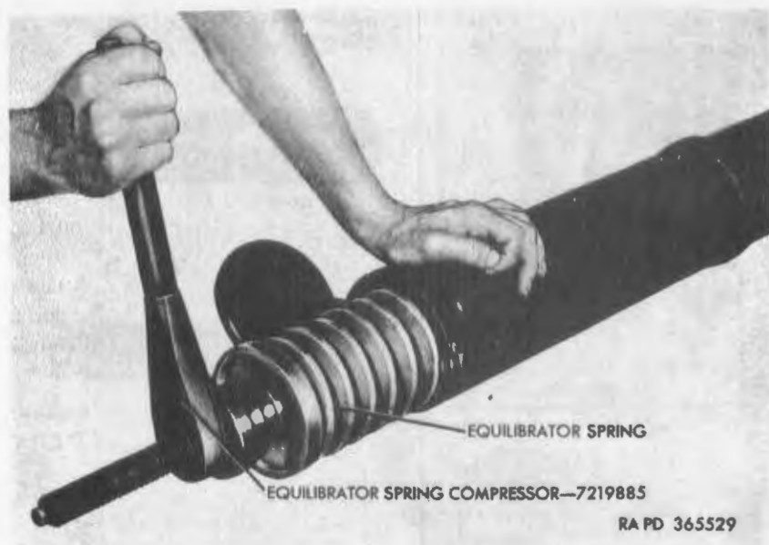
Figure 362. Removing equilibrator springs.
