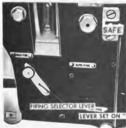
Figure 350. Three positions of firing selector lever.
