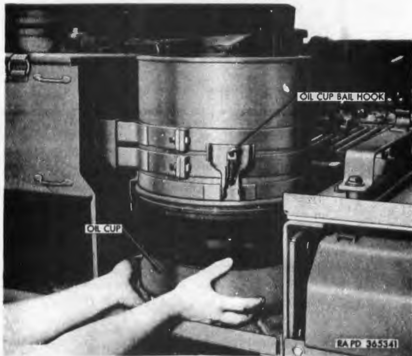
Figure 131. Removing air cleaner oil cup.
