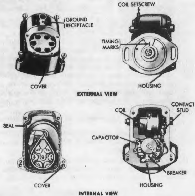
Figure 119. American Bosch magneto—separated.
