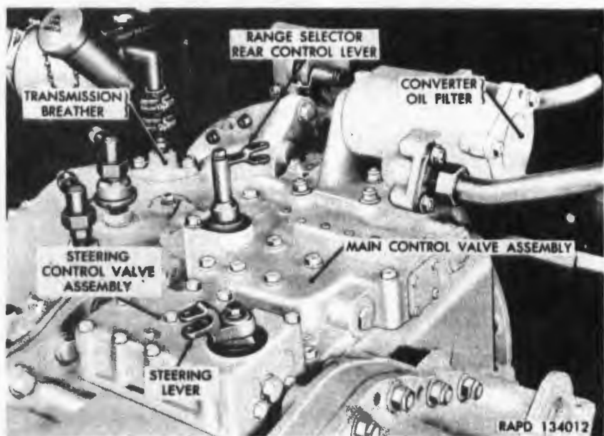
Figure 177. Transmission control valve assemblies and levers.
