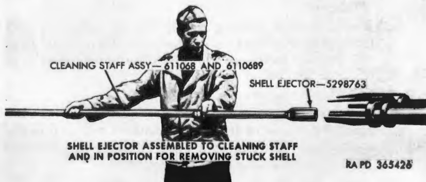
Figure 56. Removal of round using shell ejector—5298763.
