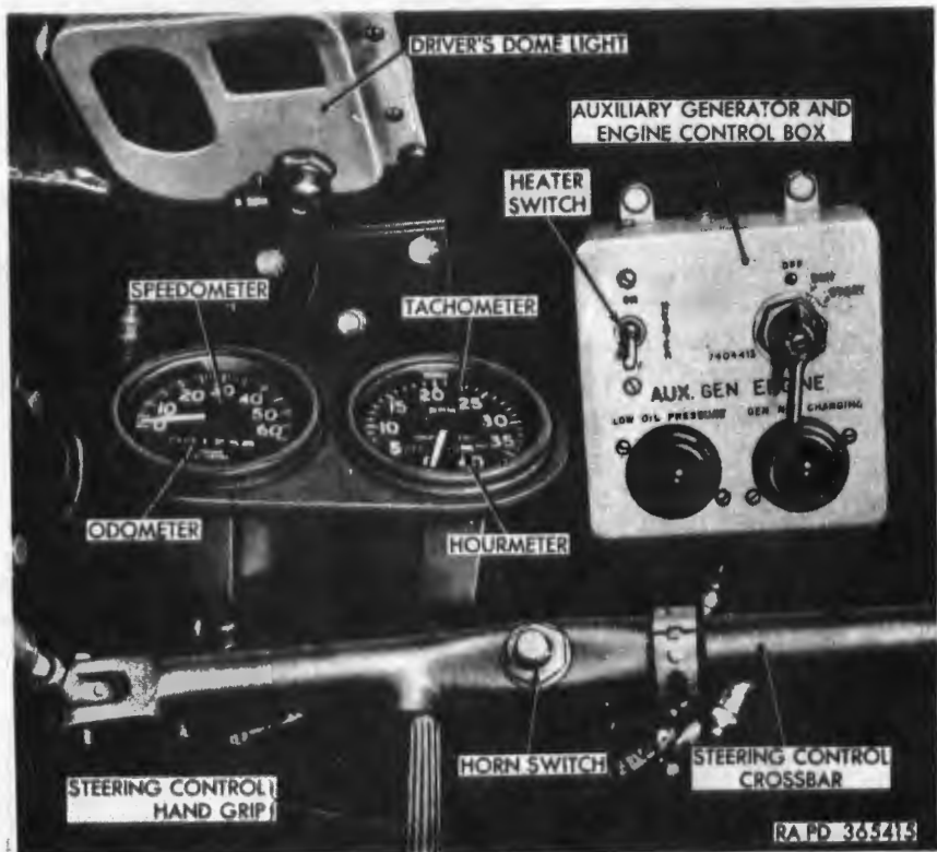
Figure 18. Speedometer, tachometer, and auxiliary generator and engine control box.
