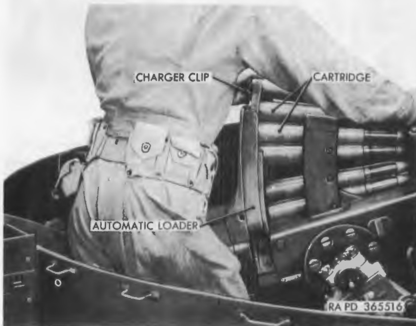
Figure 55. Loading clips of cartridges in gun.
