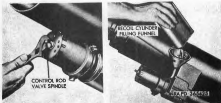
Figure 291. Filling and adjusting recoil cylinder.
