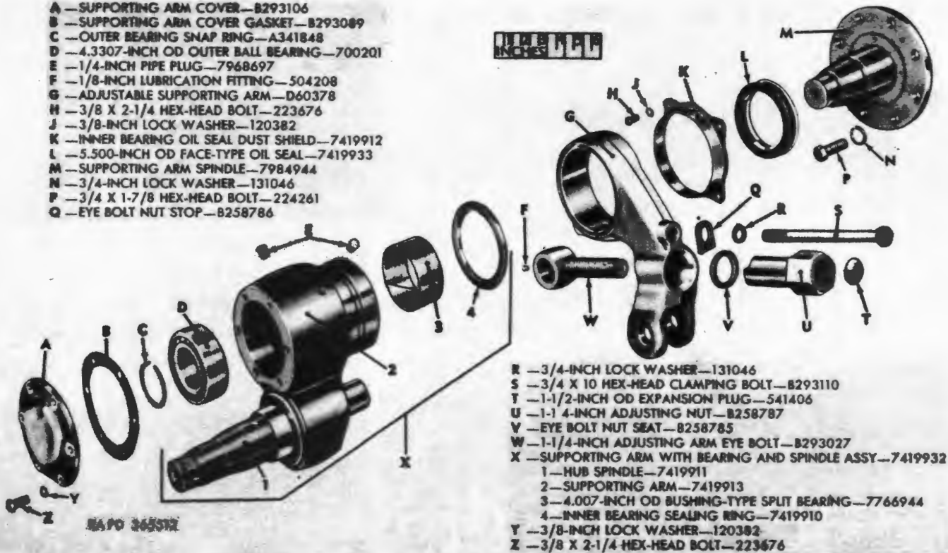
Figure 227. Compensating wheel supporting arms and supporting arm spindle—exploded view.
