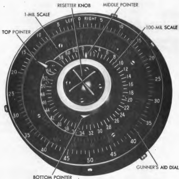
Figure 42. Azimuth indicator M27 dial.
