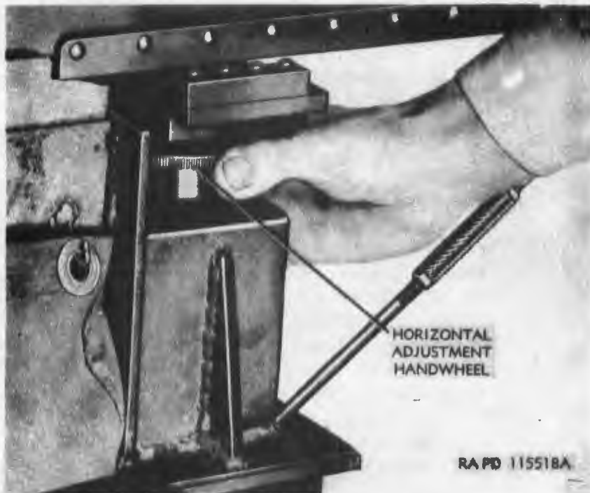
Figure 386. Adjusting subcaliber gun in azimuth.
