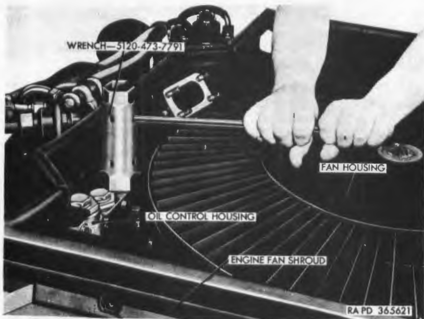
Figure 107. Removing oil pressure control valve.
