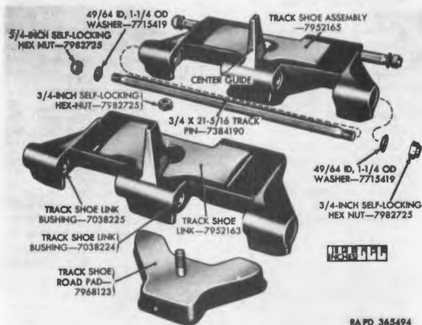
Figure 202. Track shoe assembly—exploded view.
