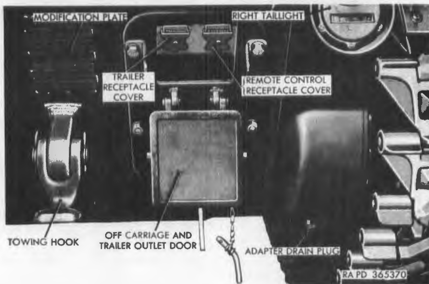
Figure 30. Remote control and trailer receptacle location.
