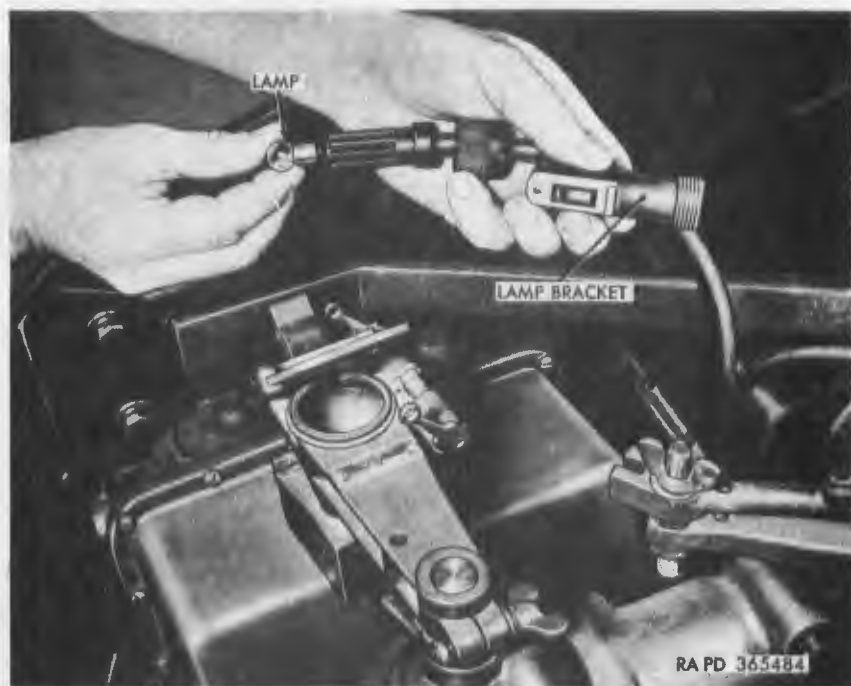
Figure 268. Replacing lamp in reflex signal light.
