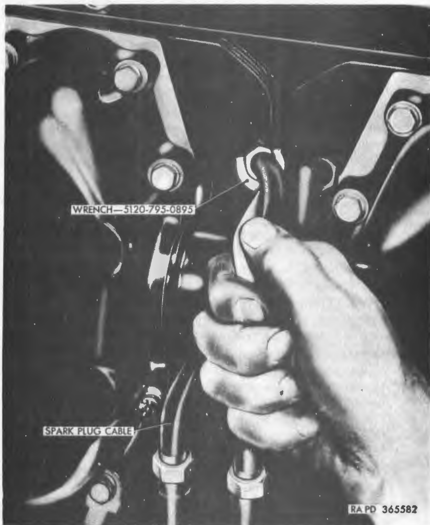
Figure 120. Removing or installing spark plug cable.
