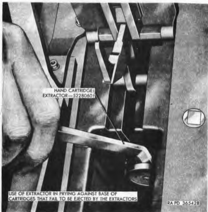
Figure 58. Removal of case, using hand cartridge extractor—5228060.
