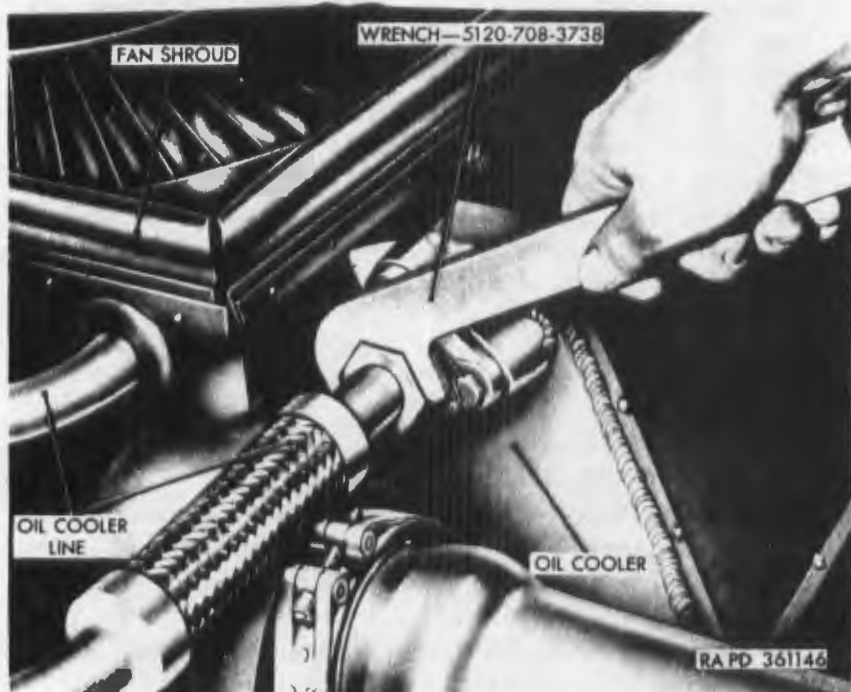
Figure 137. Removing oil cooler lines.
