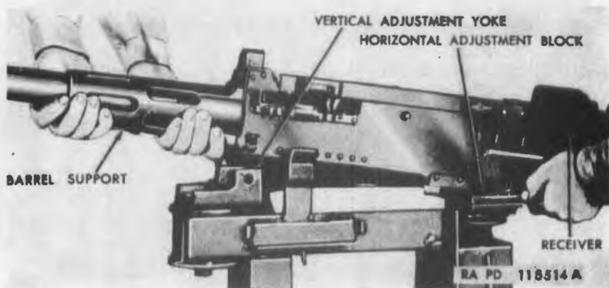
Figure 381. Installing cal..50 machine gun on the subcaliber mount.
