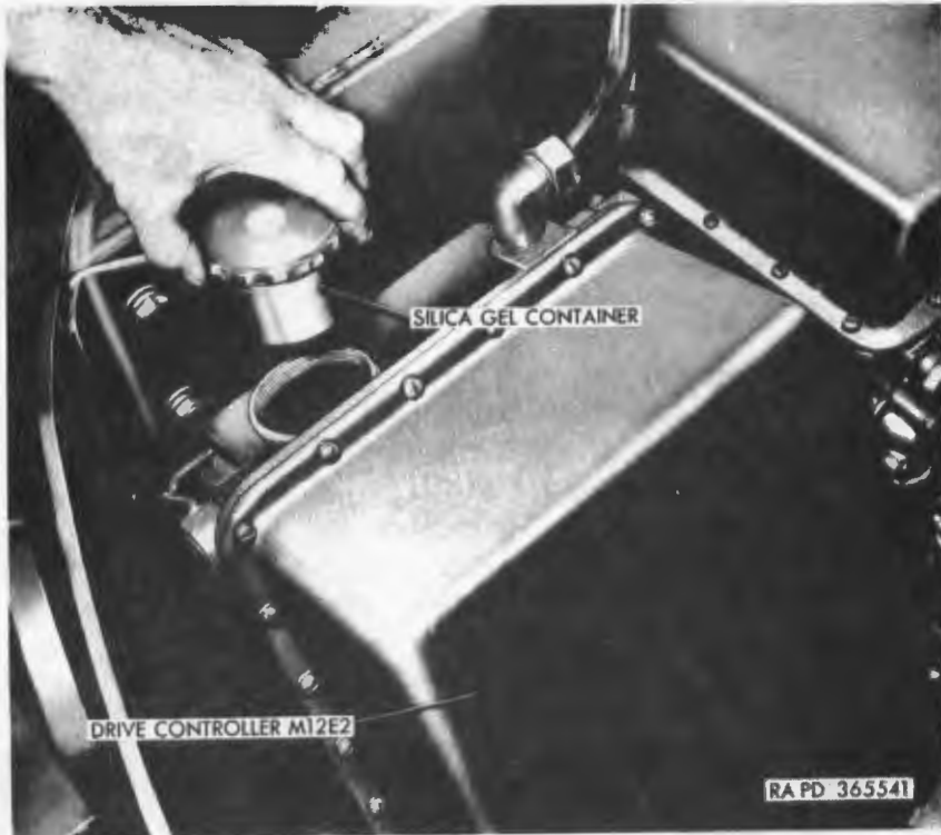
Figure 269. Replacing silica gel container in drive controller M12E2.
