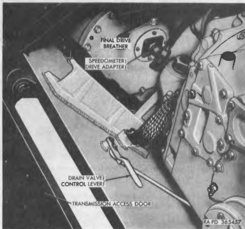
Figure 14. Engine compartment rear drain valve control lever.
