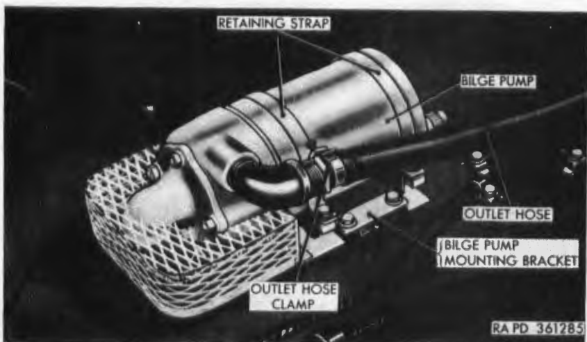
Figure 64. Engine compartment bilge pump.
