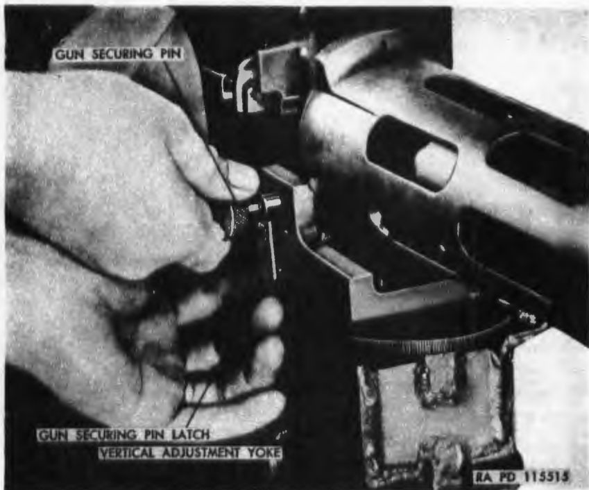
Figure 382. Inserting gun securing pin in vertical adjustment yoke.
