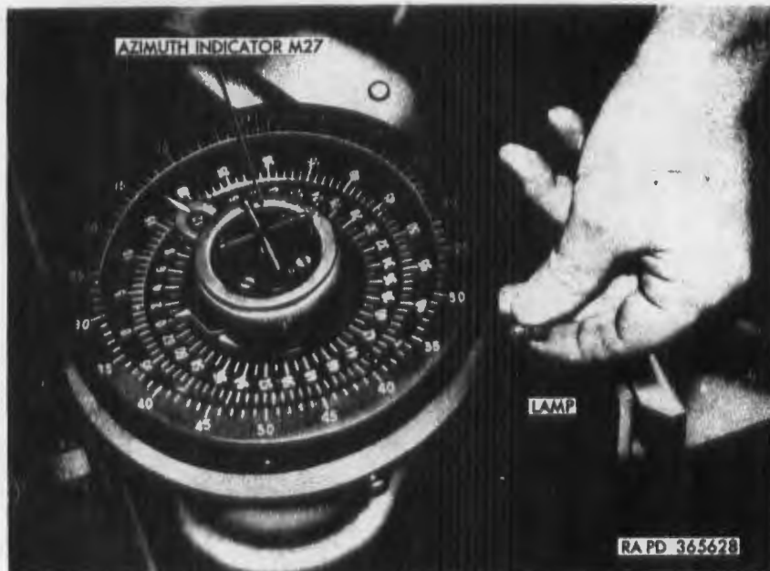
Figure 274. Replacing lamp in azimuth indicator M27.
