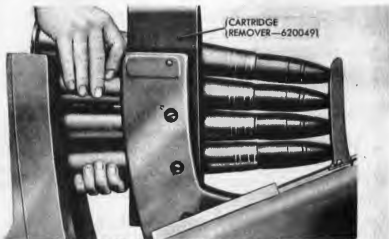
REMOVAL OF ROUNDS IN AUTOMATIC LOADER USING CARTRIDGE REMOVER
