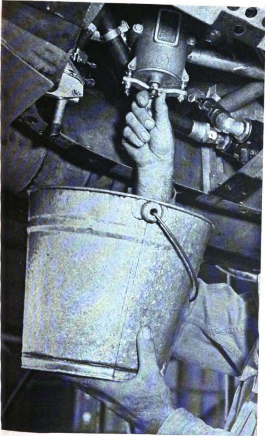
Figure 49. Draining the main-line strainer.
