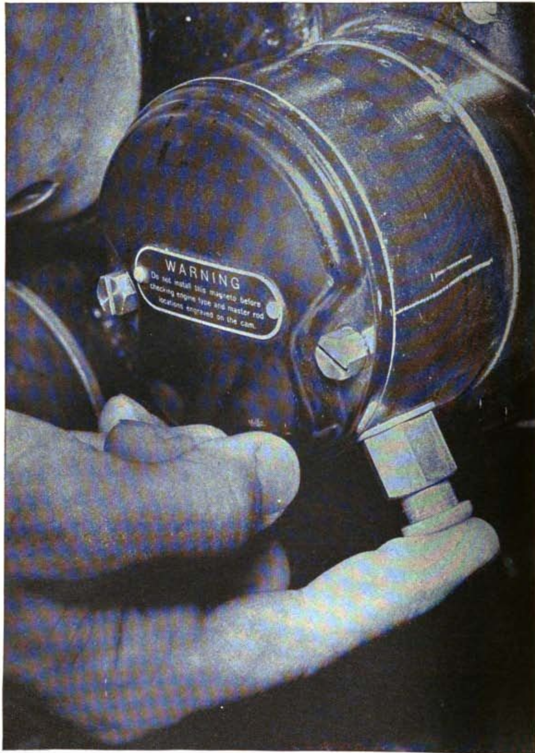
Figure 63. Oiling magneto by pressing oiler button.
