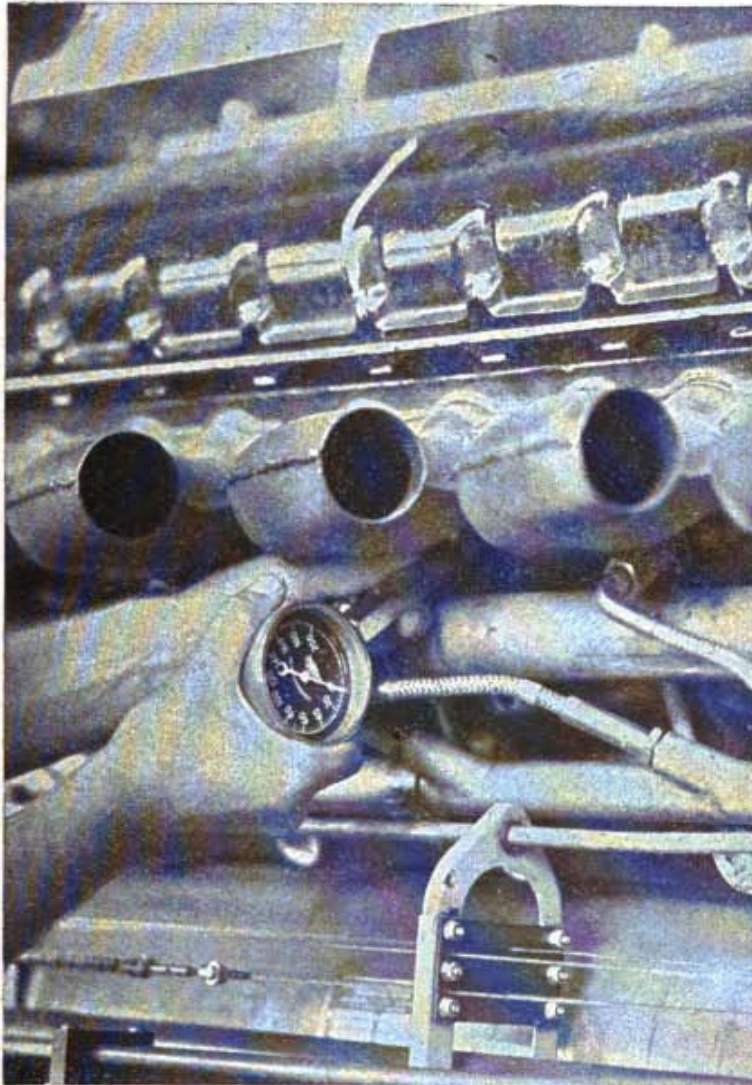
Figure 75. Checking cylinder pressure with a compression gauge.
