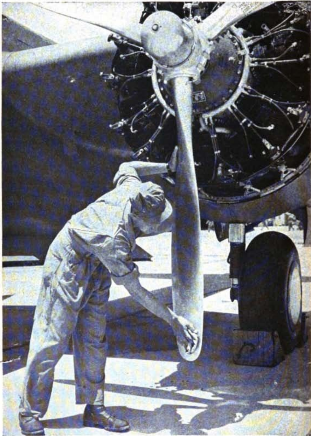
Figure 54. Coating the propeller with engine oil.
