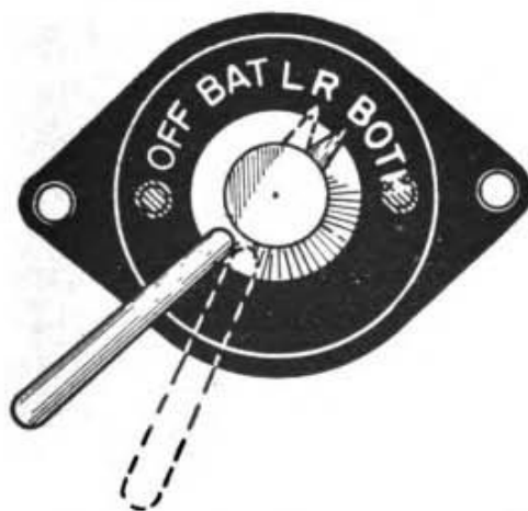
Figure 39. Checking engine operation on right magneto.
