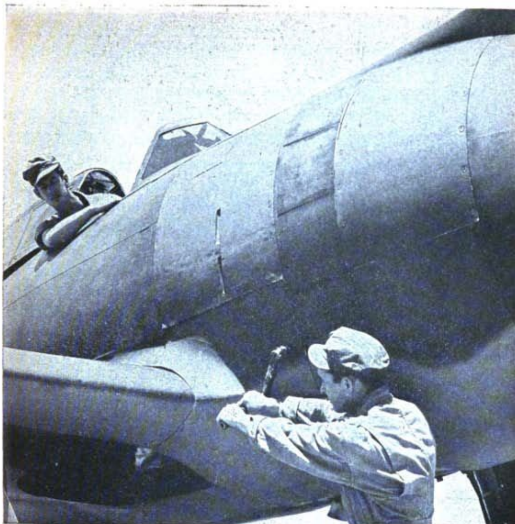
Figure 26. Energizing the starter flywheel with a hand crank.
