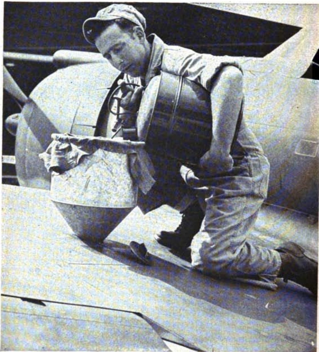
Figure 46. Using a small container for refueling.
