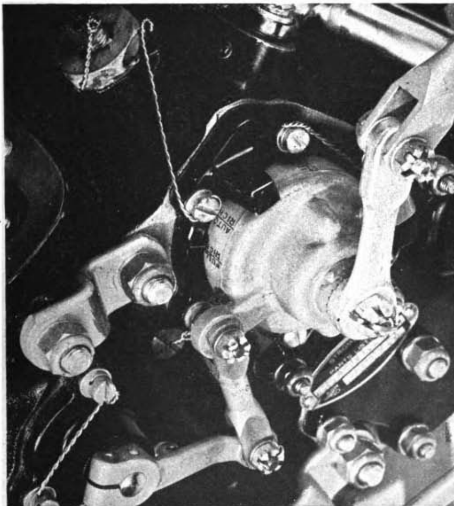
Figure 53. Mixture control in FULL RICH position (at the carburetor).
