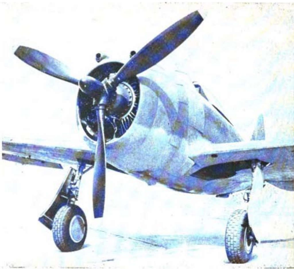
Figure 3. Radial type engine mounted in the nose.
