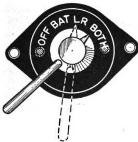
Figure 38. Checking engine operation on left magneto.
