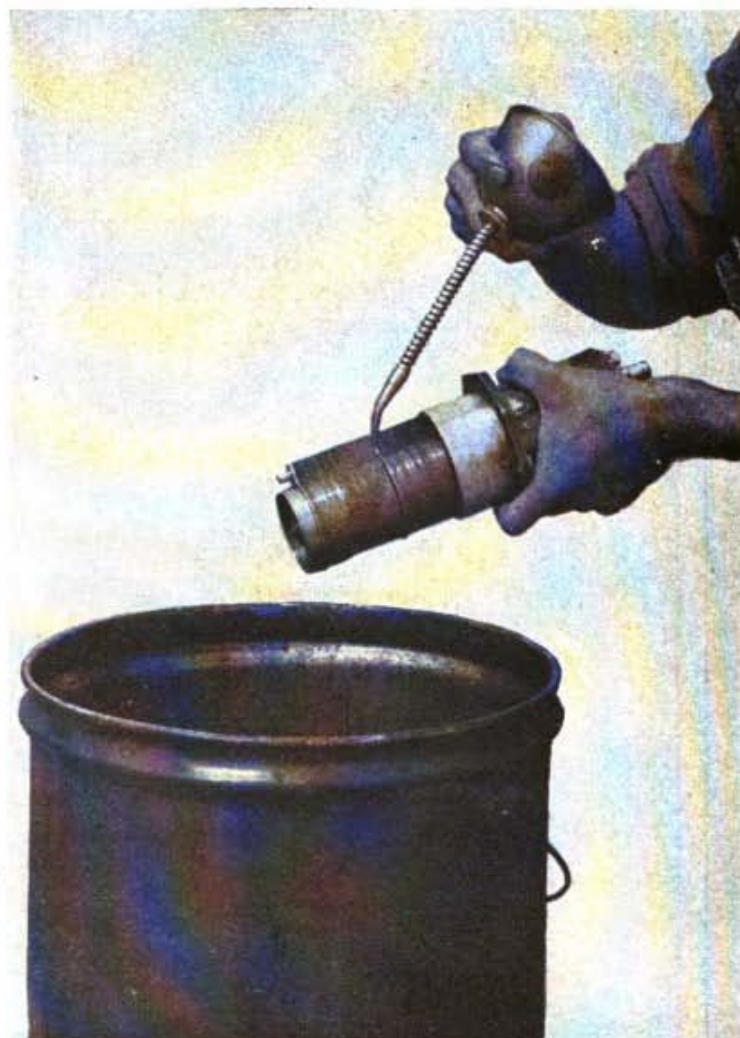
Figure 58. Coating a Cuno with engine oil before replacement.
