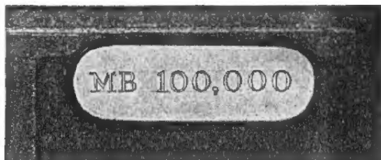
Engine Number located on right side of cylinder block front upper corner.
