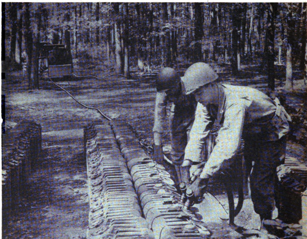
Figure 13. Method of filling 5-gallon cans using 100-gallon-per-minute dispenser.
