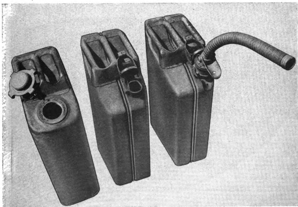
Figure 3. Five-gallon gasoline cans ("ameri-can," "jerrican," and "jerrican" with adapter and flexible nozzle).
