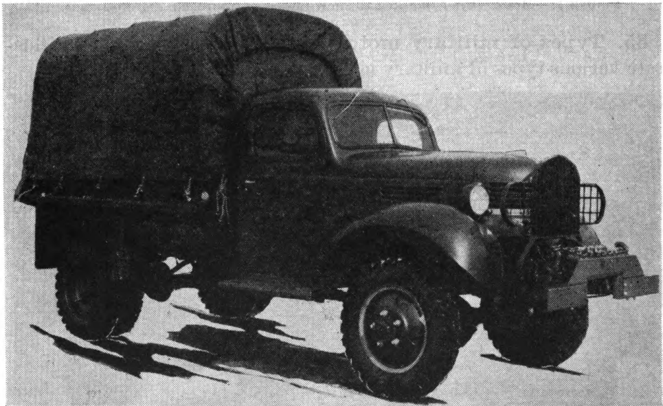
FIGURE 4.—Truck, 1½-ton, 4 x 4 (2dt), cargo (closed cab), Dodge 1940, with front end mounted winch (type 3 vehicle).
