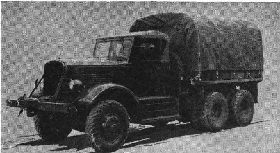
FIGURE 6.—Truck, 4-ton, 6 x 4 (4dt), cargo (open cab), Autocar 1940, with front end mounted winch (type 4 vehicle).
