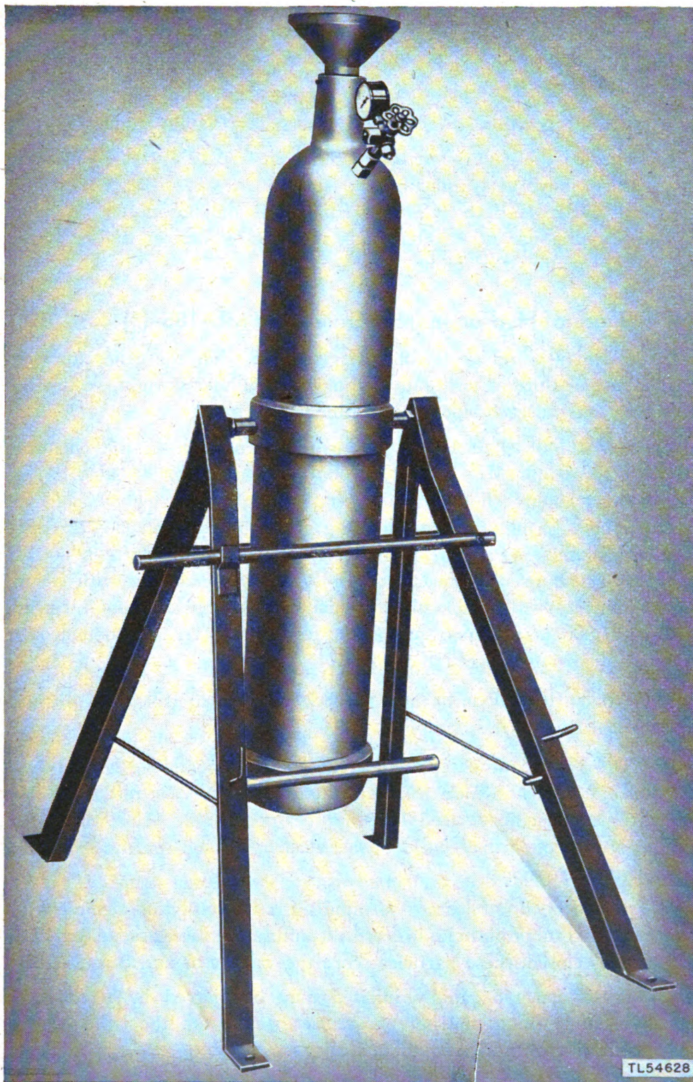
Figure 11. Generator ML-185-B in upright charging position.
