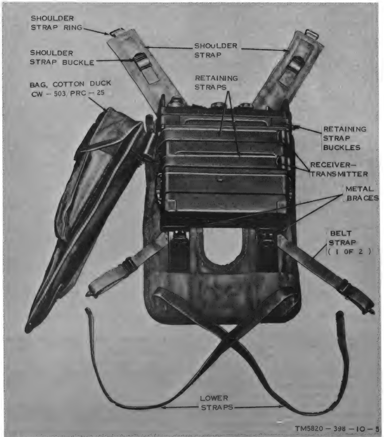
Figure 2-3. Installation of receiver-transmitter in ST-138/PRC-25.
