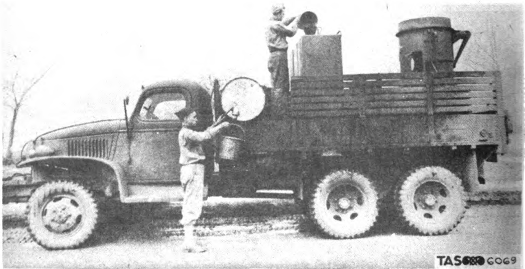
Fig. 69. Filling Special Oil Supply Tank by Hand.
