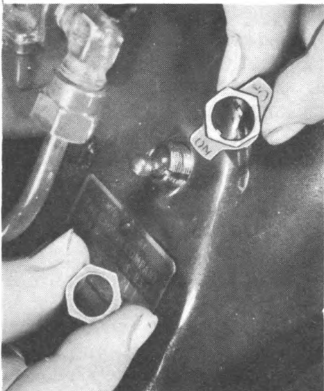
Fig 42. Ignition switch hex nut and lock washer detached from flywheel housing.
