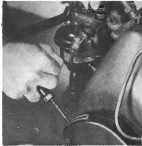
Fig 22. Manipulating ready pull-starter and choke to start engine.
