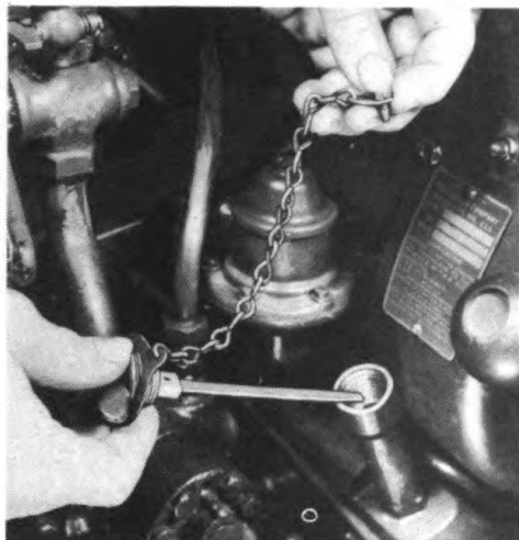
Fig 44. Removing crankcase filler cap to permit loosening of one flywheel housing cap screw.
