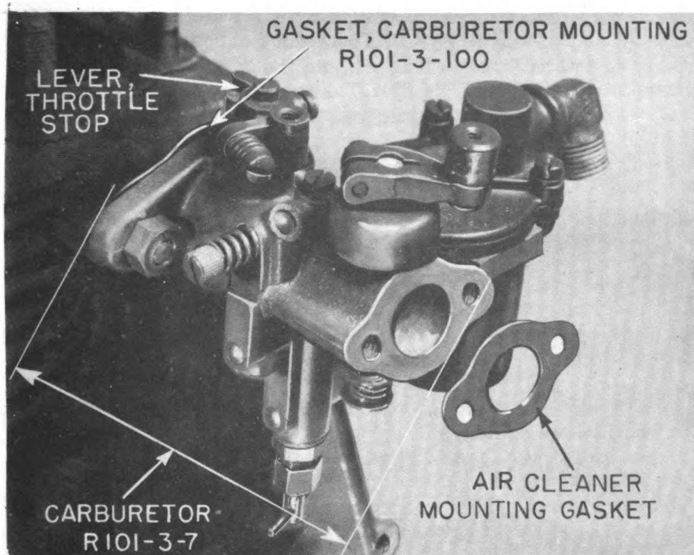
Fig 55. Carburetor, showing Chemical Warfare Service nomenclature of parts.
