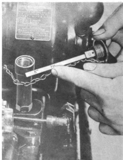
Fig 34. Checking crankcase oil level.
