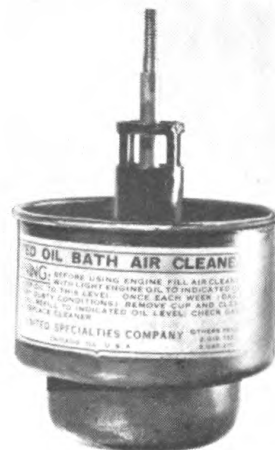
Fig 30. Oil bath air cleaner disassembled.
