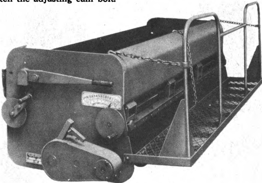
Plate No. 14—Safety Platform for Shoveler
