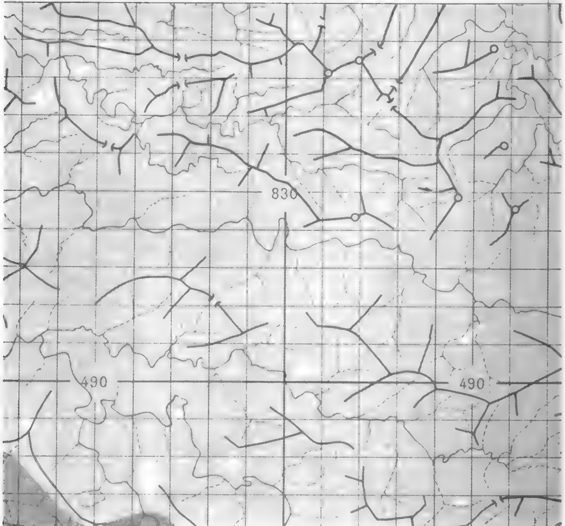
Figure 43. Section of Sheet No. 191E of the Carte de l'Indochine 1:100,000 series by the Service Géographique de l'Indochine showing relief by ridge lines.
