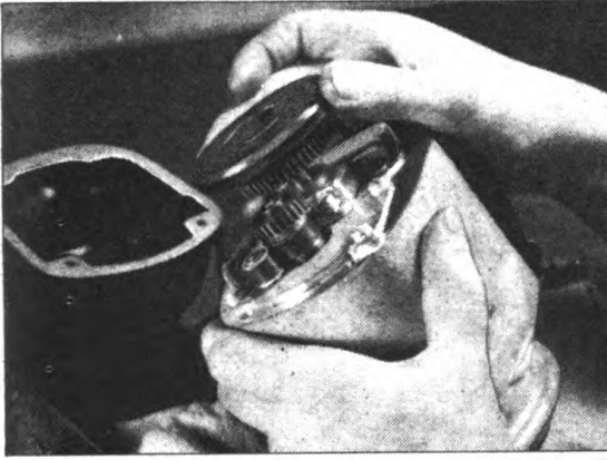
Fig. 43. Method of Removing or Properly Meshing Distributor Gear with Steel Gear
