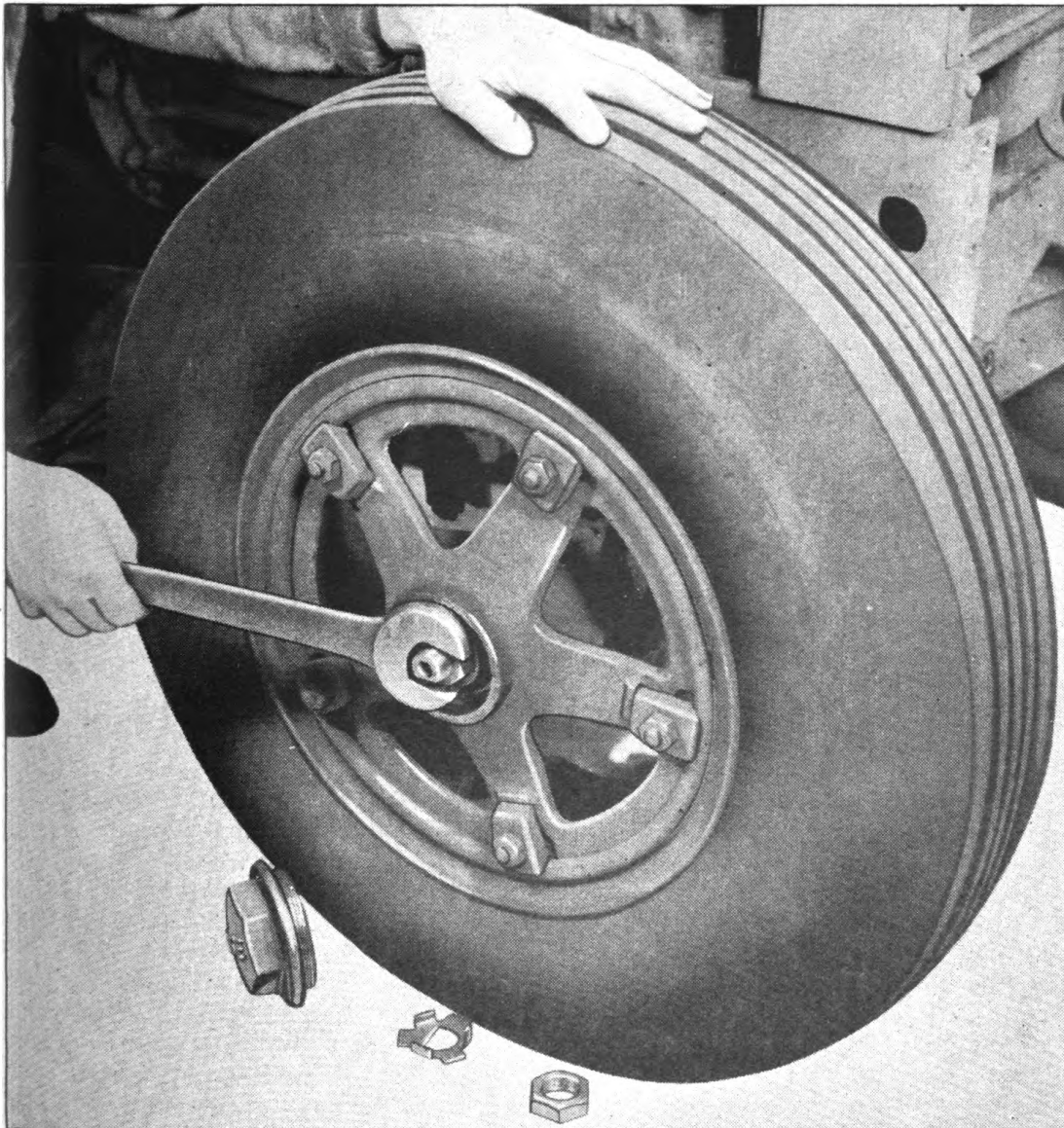
Fig. 92. Adjusting Front Wheel Bearing
