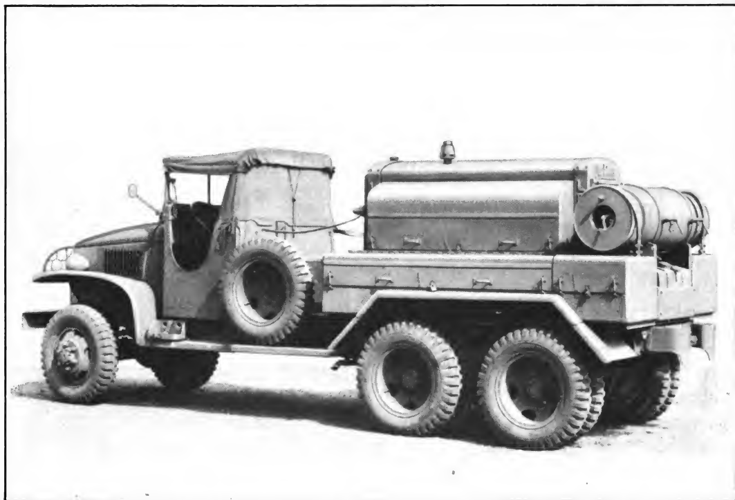
Le Roi Air Compressor Model 105GA as Mounted on GMC, 2½ Ton, 6X6 Ordnance Truck
