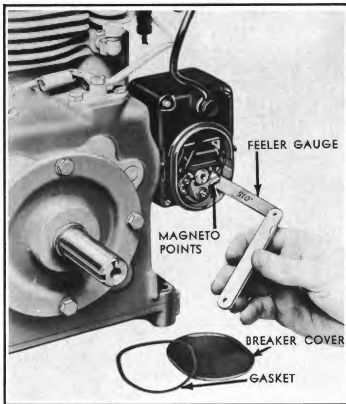
FIG. 15 Checking Magneto Breaker Points
