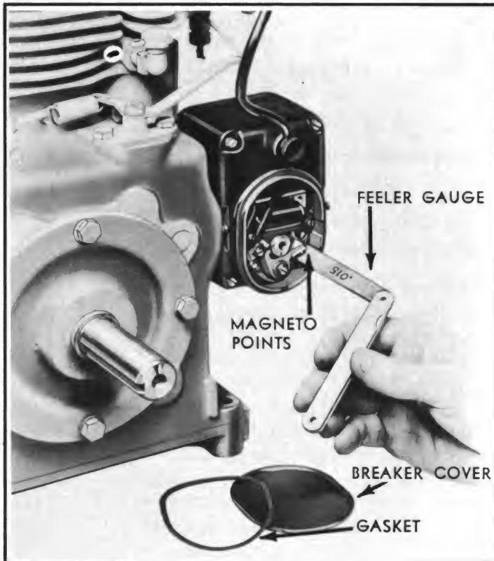
FIG. 40 Checking Magneto Breaker Points
