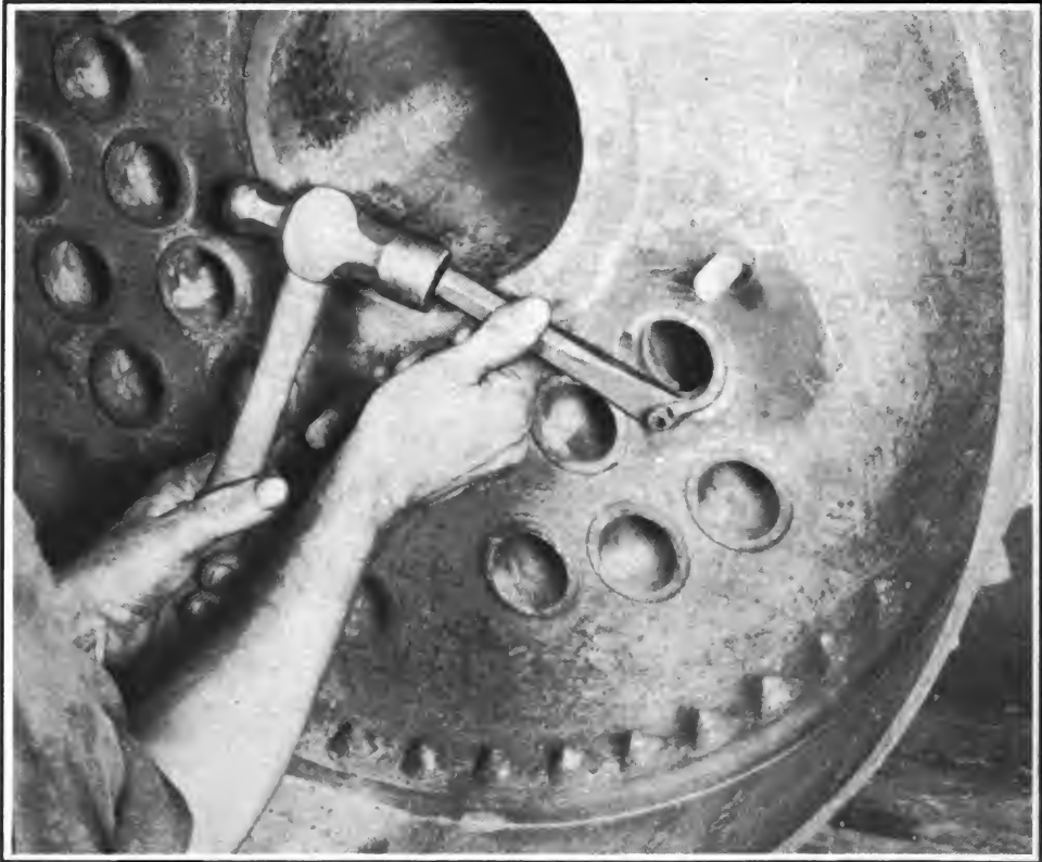
FIG. 56 Removing Bead and Weld From Tube End
