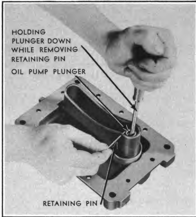
FIG. 112 Disassembly of Oil Pump
