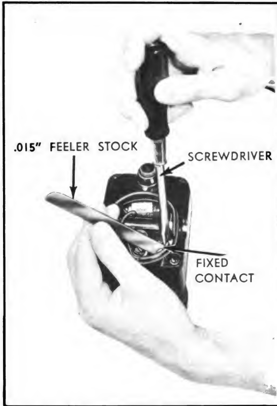
FIG. 134 Breaker Point Adjustment
