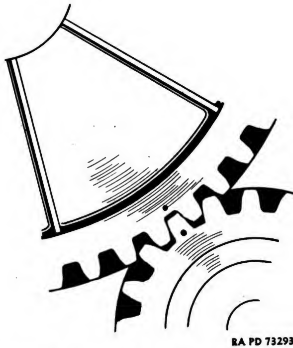
Figure 63 – Proper Meshing of Crankshaft and Camshaft Gears
