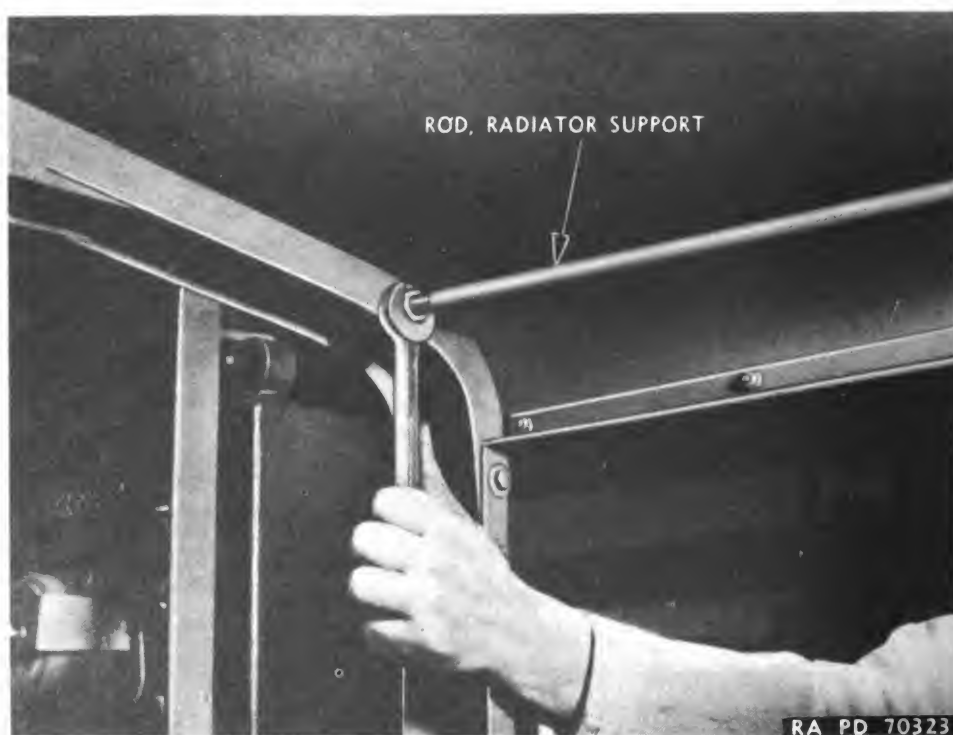
Figure 11 – Radiator Support Rod Installation
