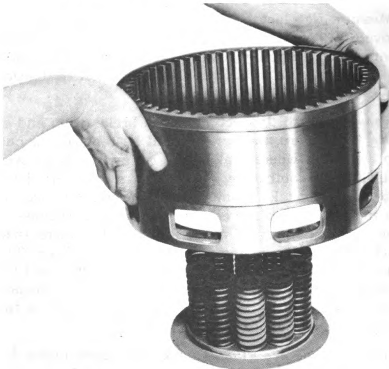
Figure 138 — Installing Brake Drum over Shifter Plate and Springs
