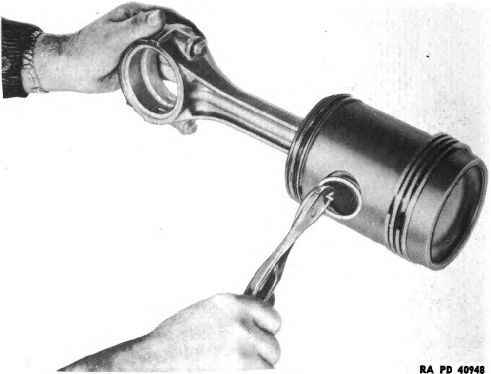
Figure 83 — Removing Lock Ring from Piston
