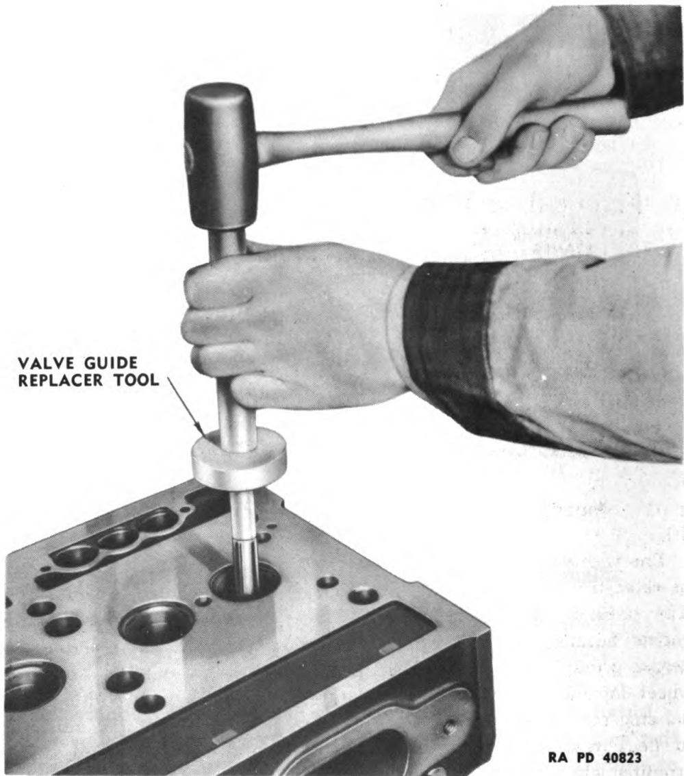
Figure 102 — Installation of Valve Guides
