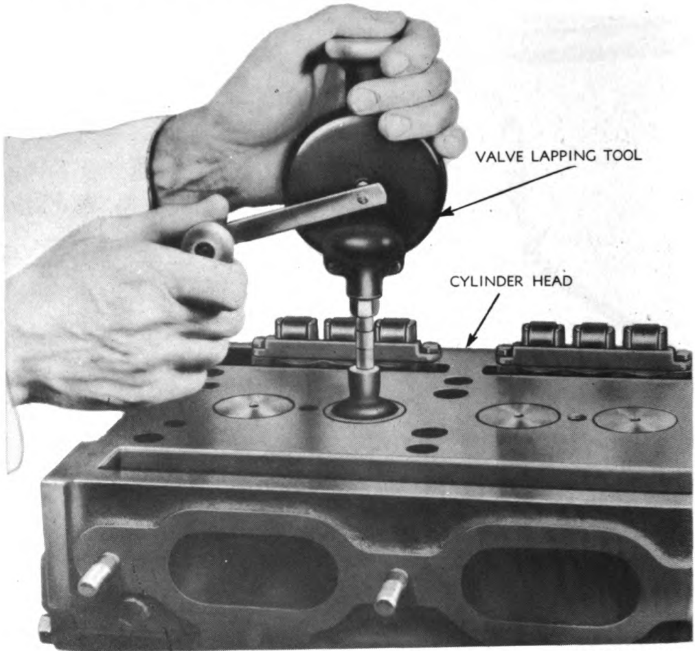
Figure 107 — Lapping Valve and Seat
