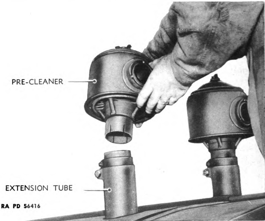
Figure 6 — Removal of Precleaners
