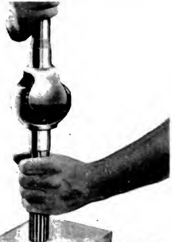
2—DISLODGING DRIVE THRUST BALL PIN
