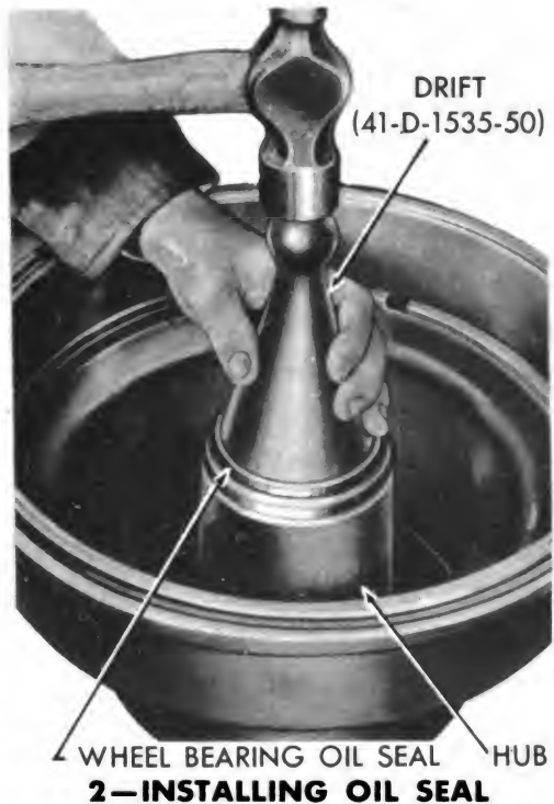
Figure 62—Conditioning and Installing Rear Wheel Bearing Oil Seal
