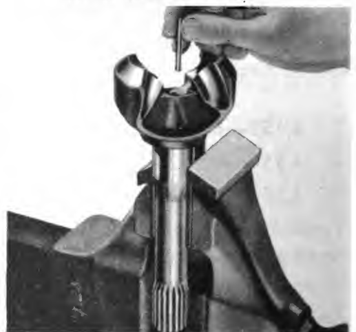
6—INSTALLING DRIVE THRUST BALL PIN
