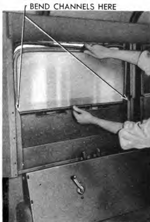
4—REMOVING SIDE WINDOW GLASS
