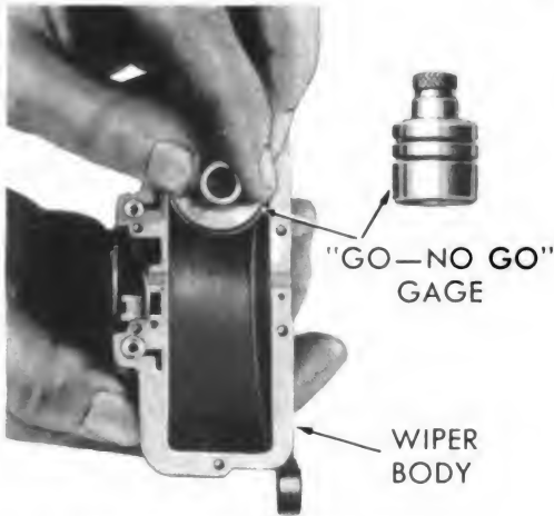
1—CHECKING WIPER BODY WITH "GO-NO GO" GAGE
