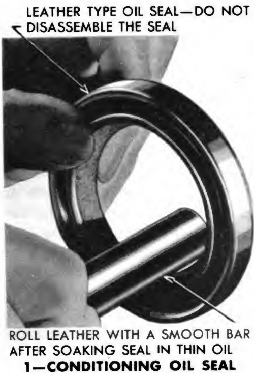
Figure 62—Conditioning and Installing Rear Wheel Bearing Oil Seal
