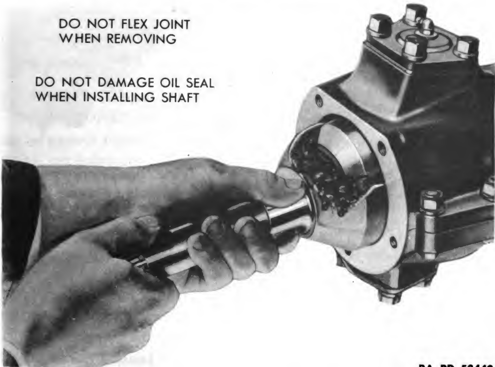
Figure 48—Removing Universal Drive Shaft
