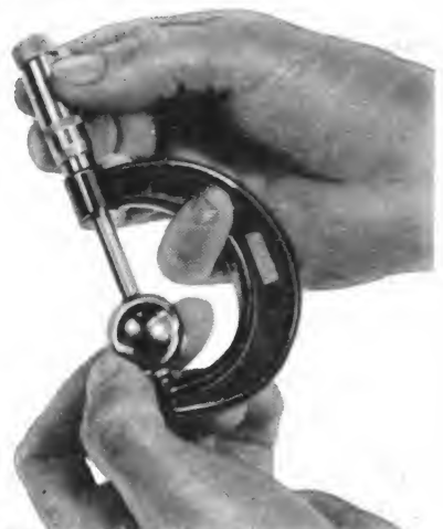
4—MEASURING DRIVE BALLS WITH MICROMETER
