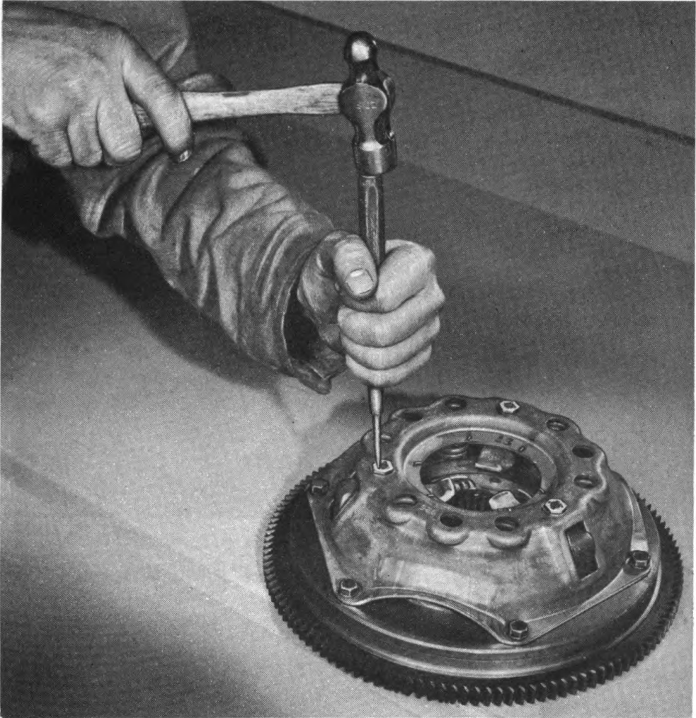
Figure 87—Locking Release Lever Adjusting Nut
