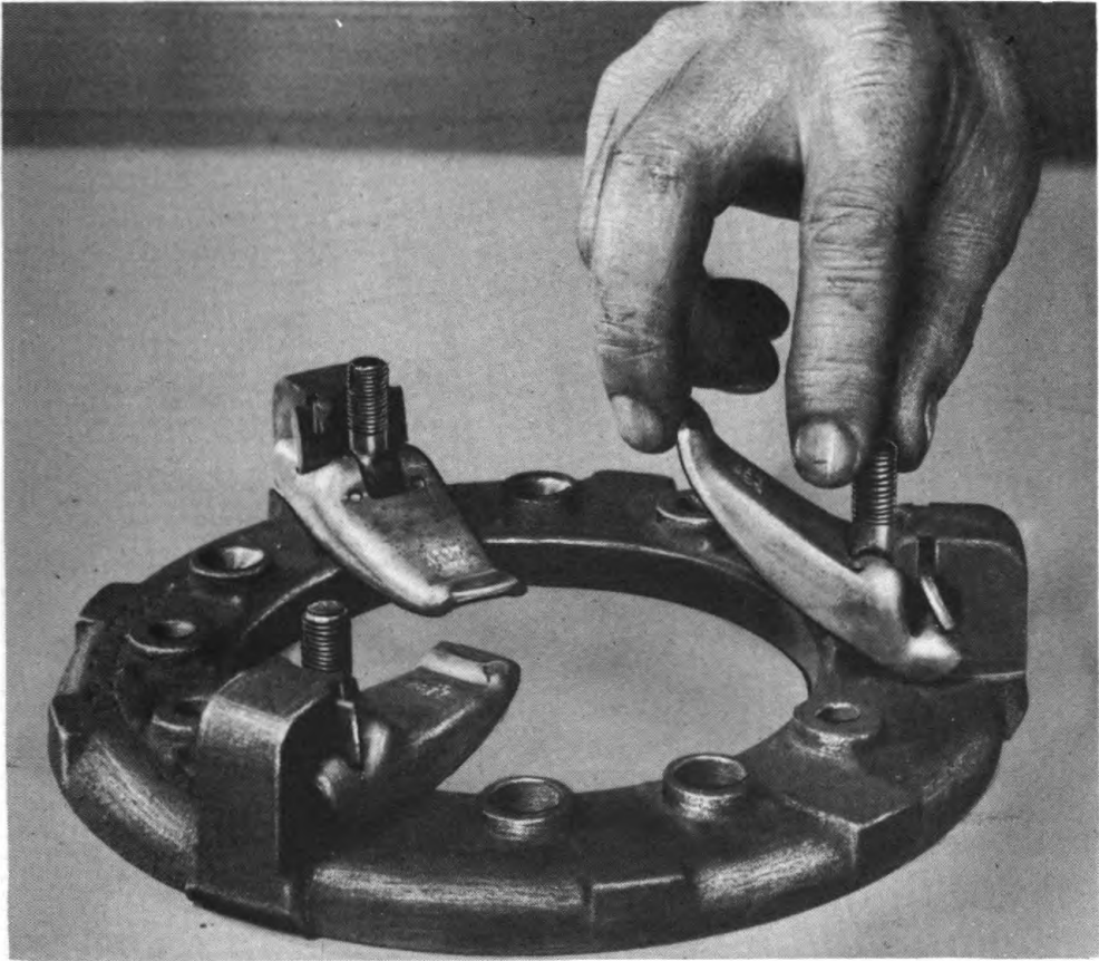
Figure 84—Removing or Installing Release Lever in Eyebolt
