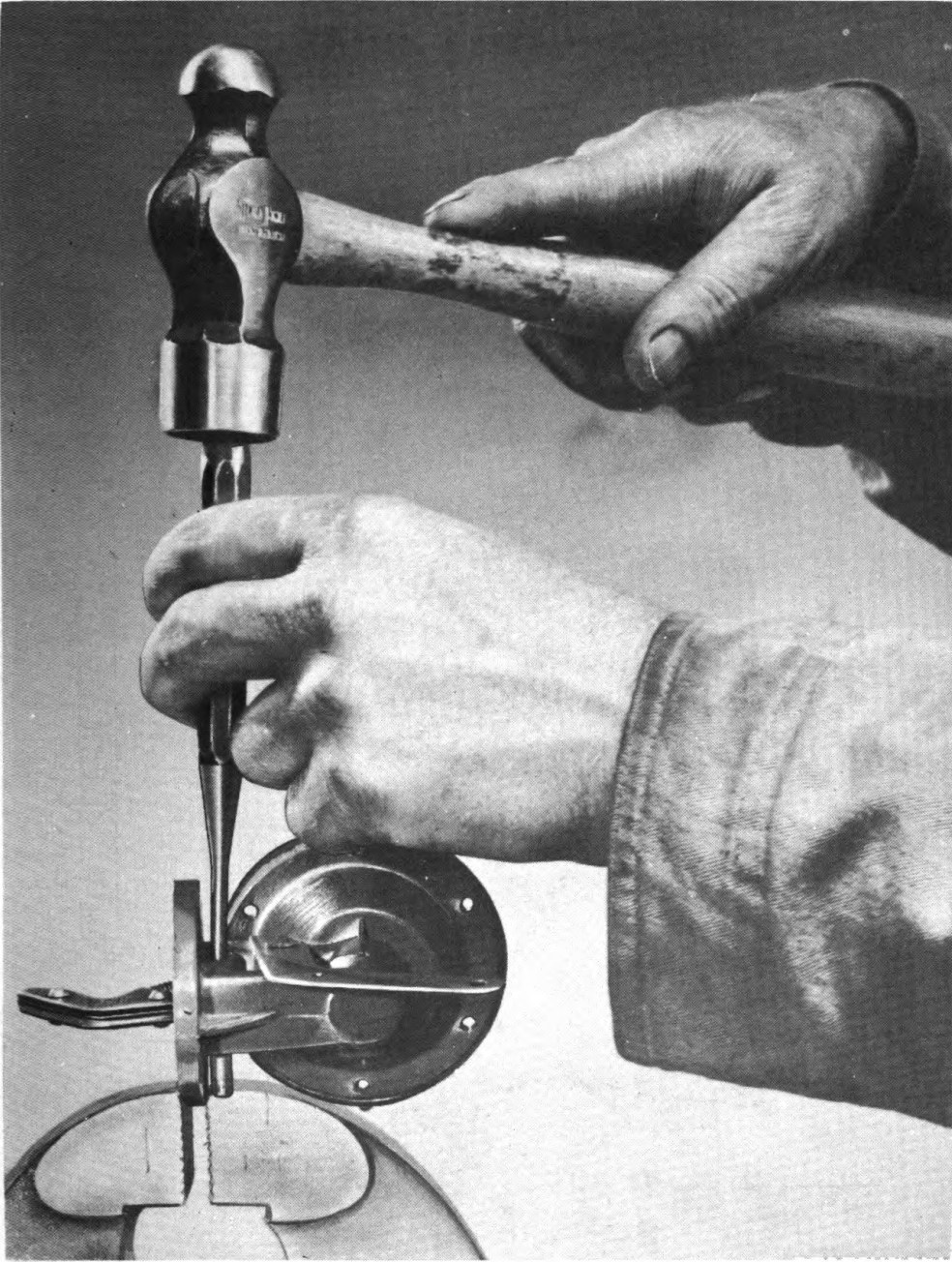
Figure 63—Removing Fuel Pump Anchor Pin and Arm
