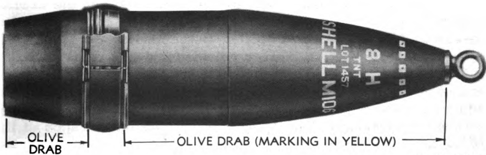
Figure 104—200-lb HE Shell M106 for 8-inch Howitzer M1
