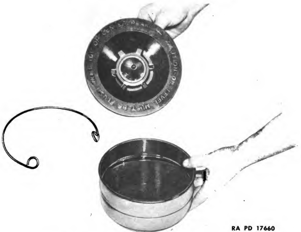
Figure 83—Removing Baffle and Baffle Ring
