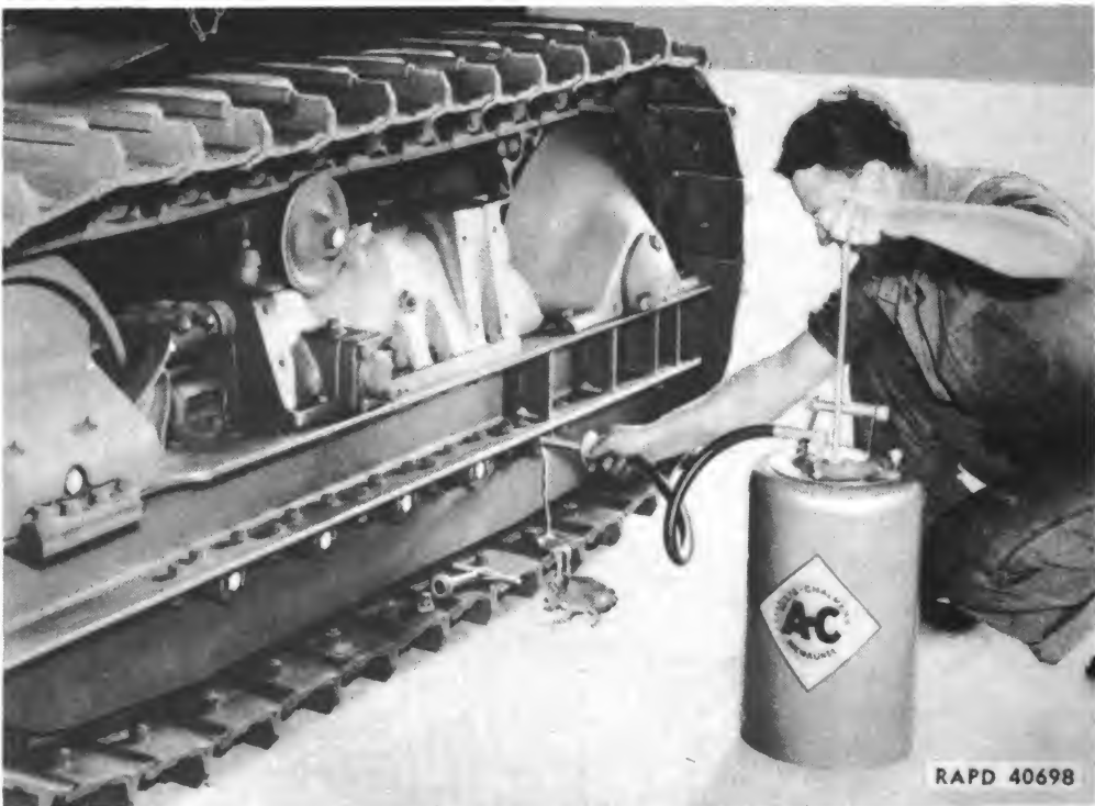
Figure 25—Lubricating Truck Wheels
