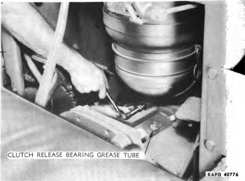
Figure 44—Removing Cap Screw Holding Engine to Spacer
