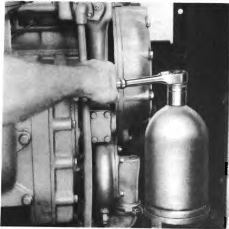
Figure 94—Removing Lubricating Oil Filter Stud
