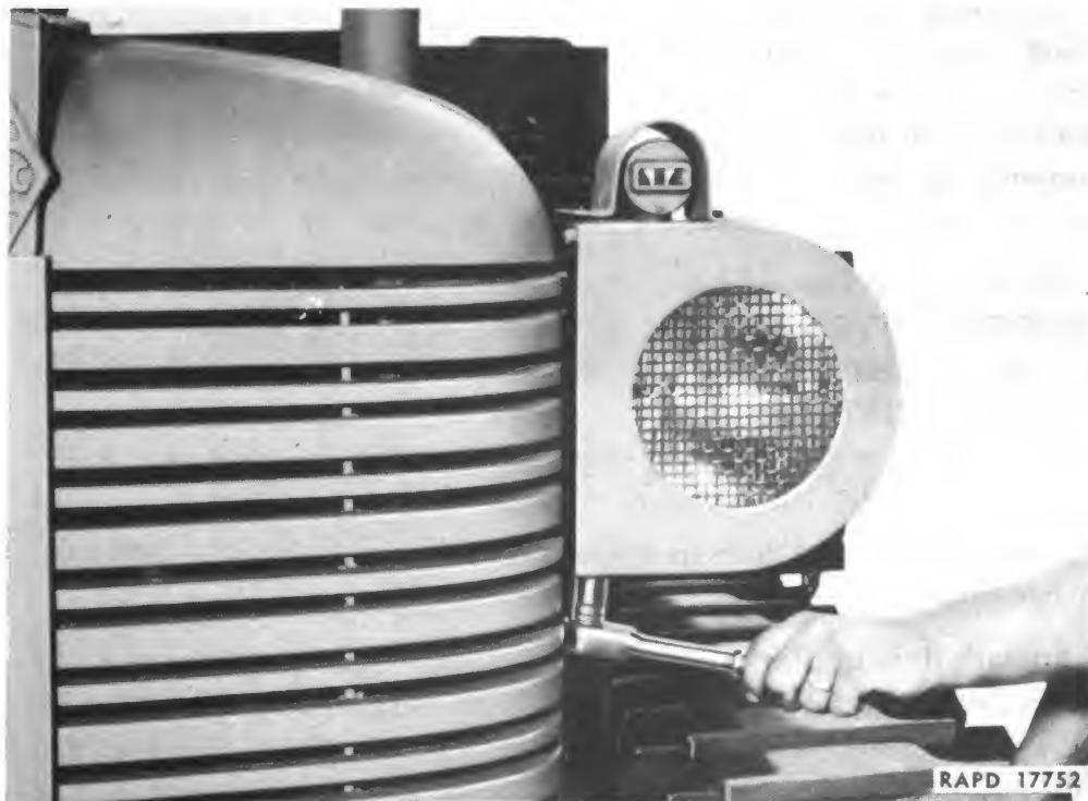
Figure 109—Removing Headlight Guard
