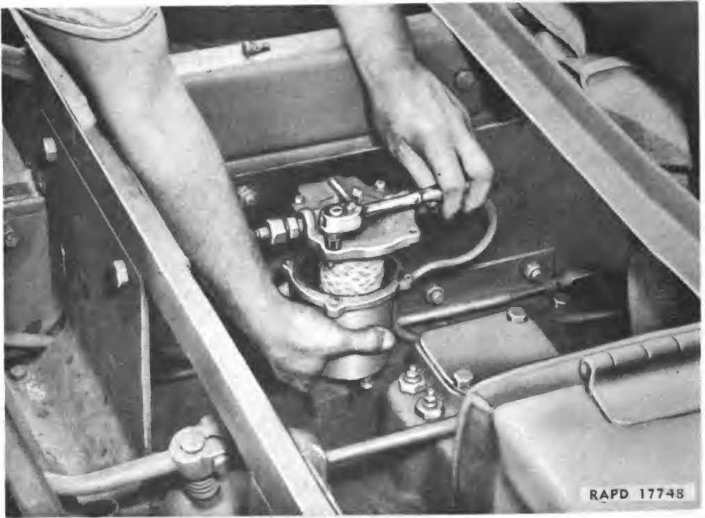
Figure 59—Removing First Stage Fuel Filter Cup
