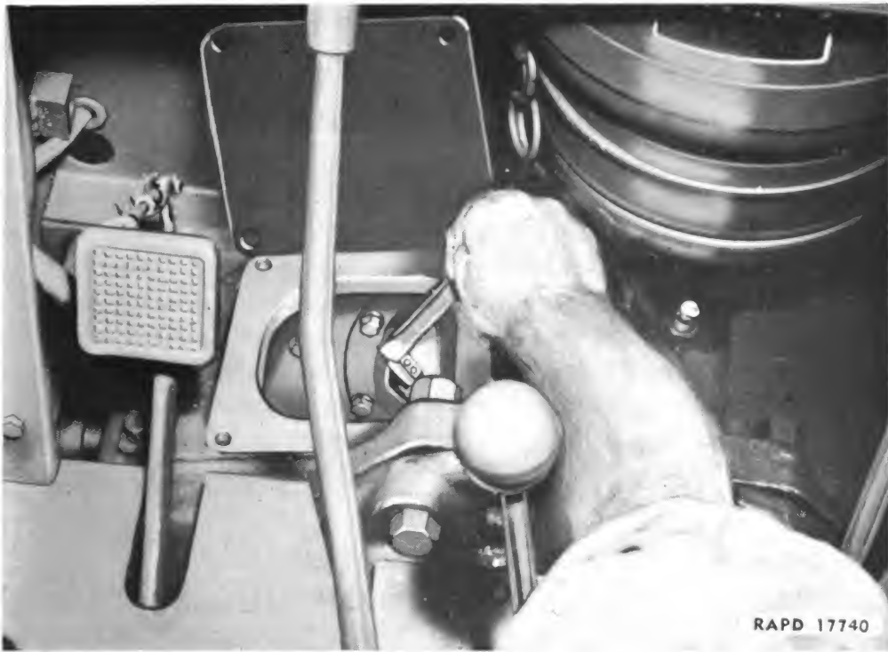
Figure 116—Adjusting Master Clutch
