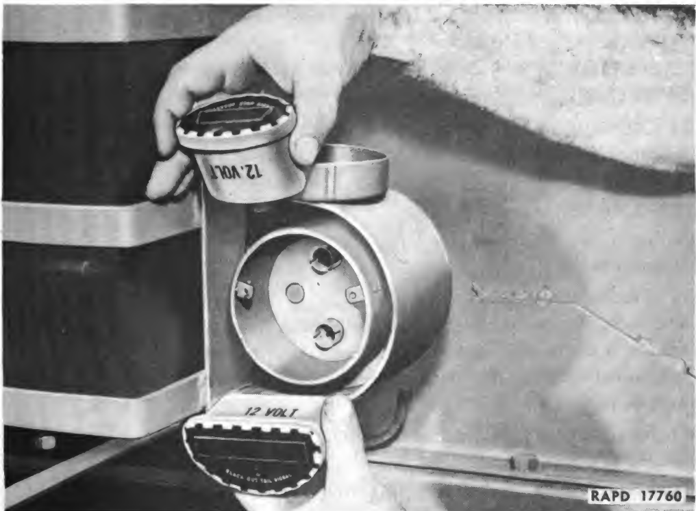
Figure 113—Removing Lamp Units from Taillight
