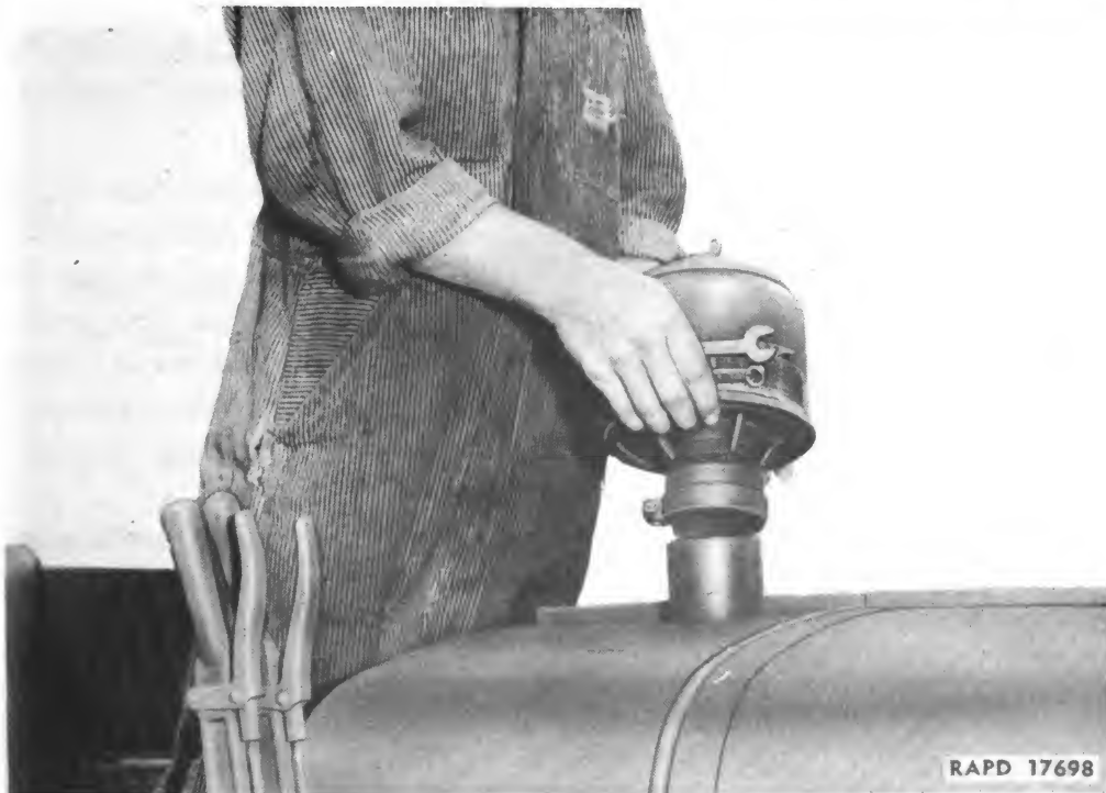
Figure 81—Removing Air Precleaner
