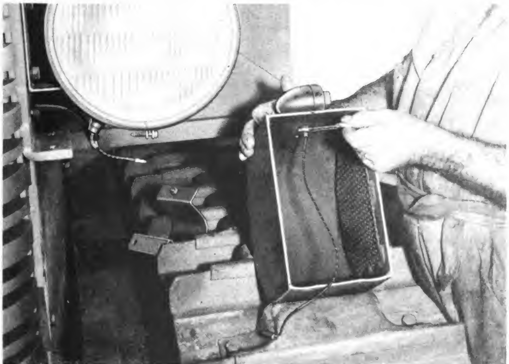
Figure 111—Removing Blackout Headlight
