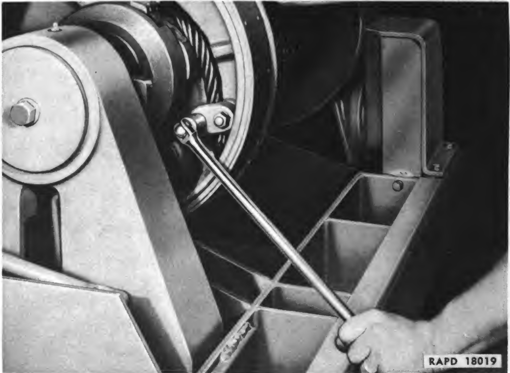
Figure 134—Removing Cable Clamp
