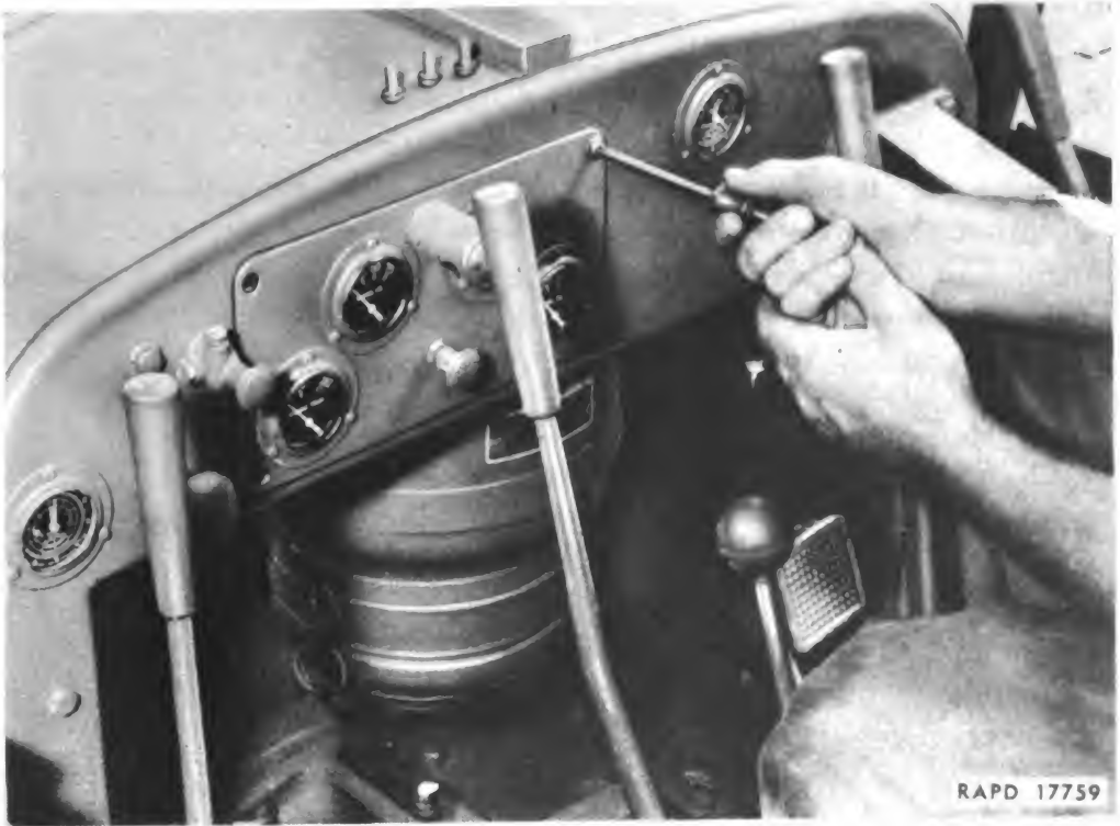
Figure 104—Removing Screws from Instrument Panel
