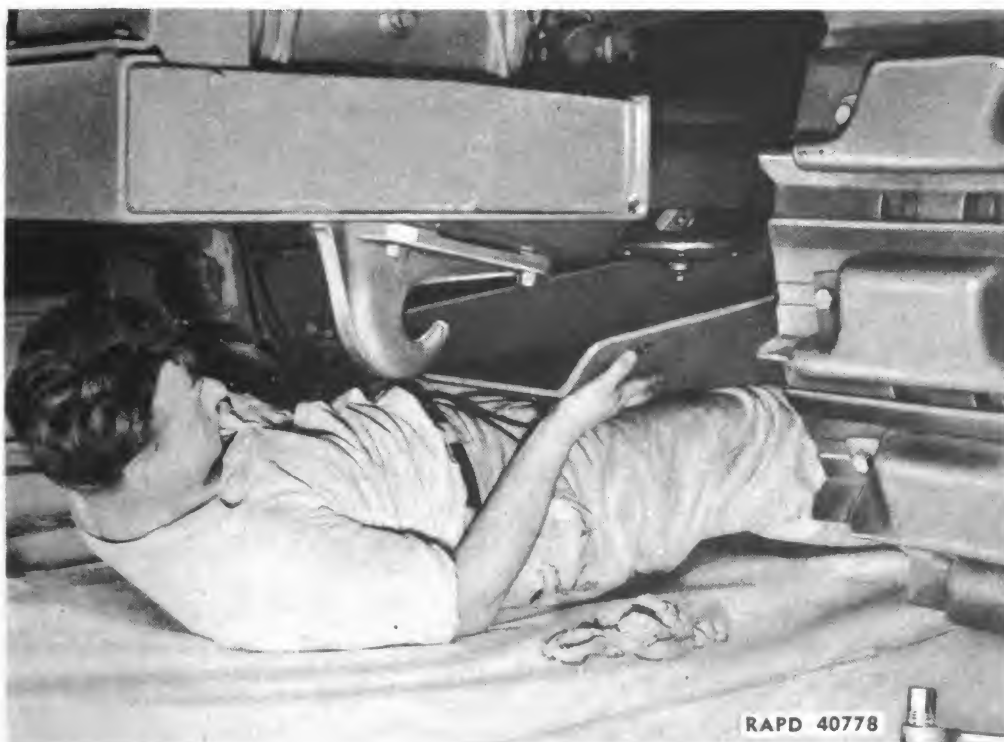
Figure 97—Removing Engine Support Bottom Cover
