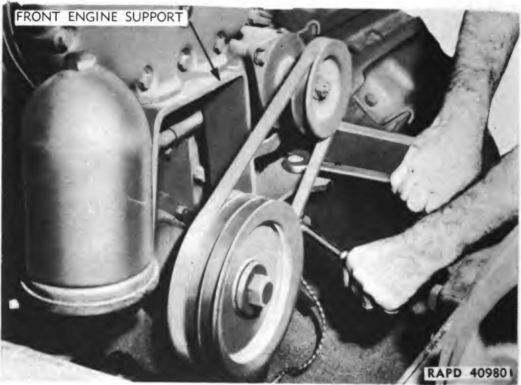
Figure 43—Removing Bolts from Front Engine Support
