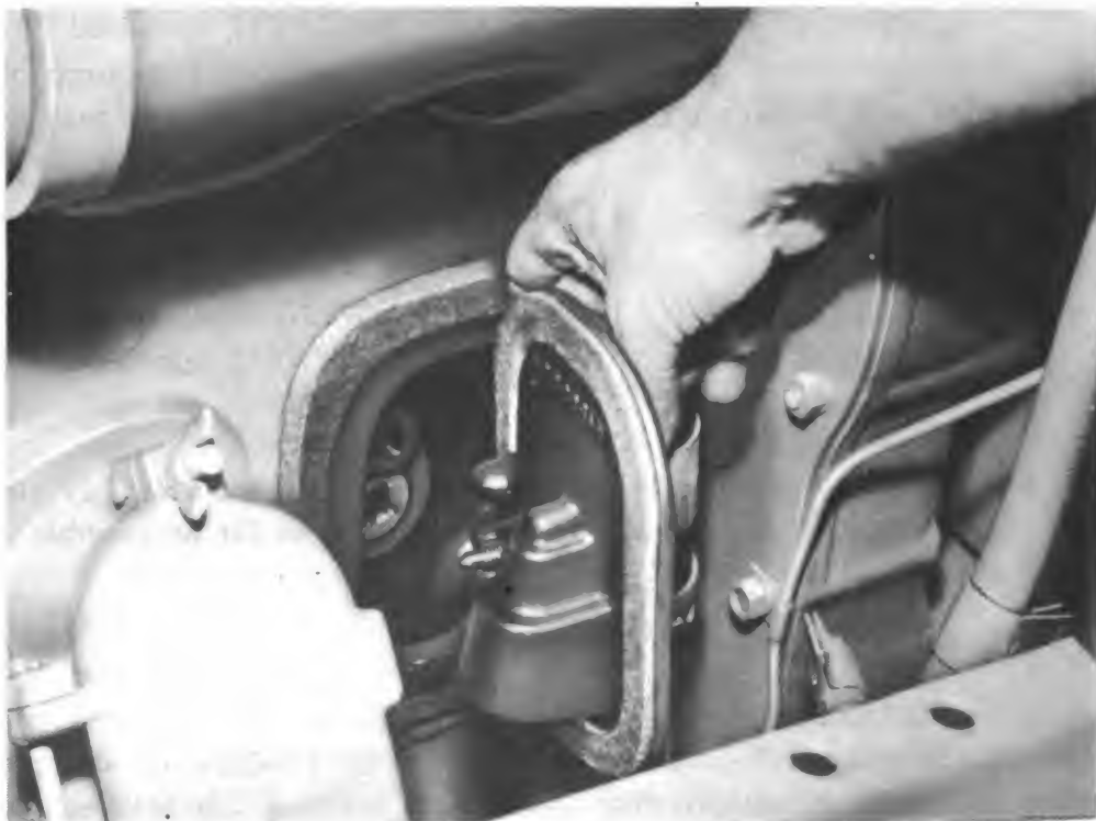
Figure 107—Removing Air Heater Burner Unit
