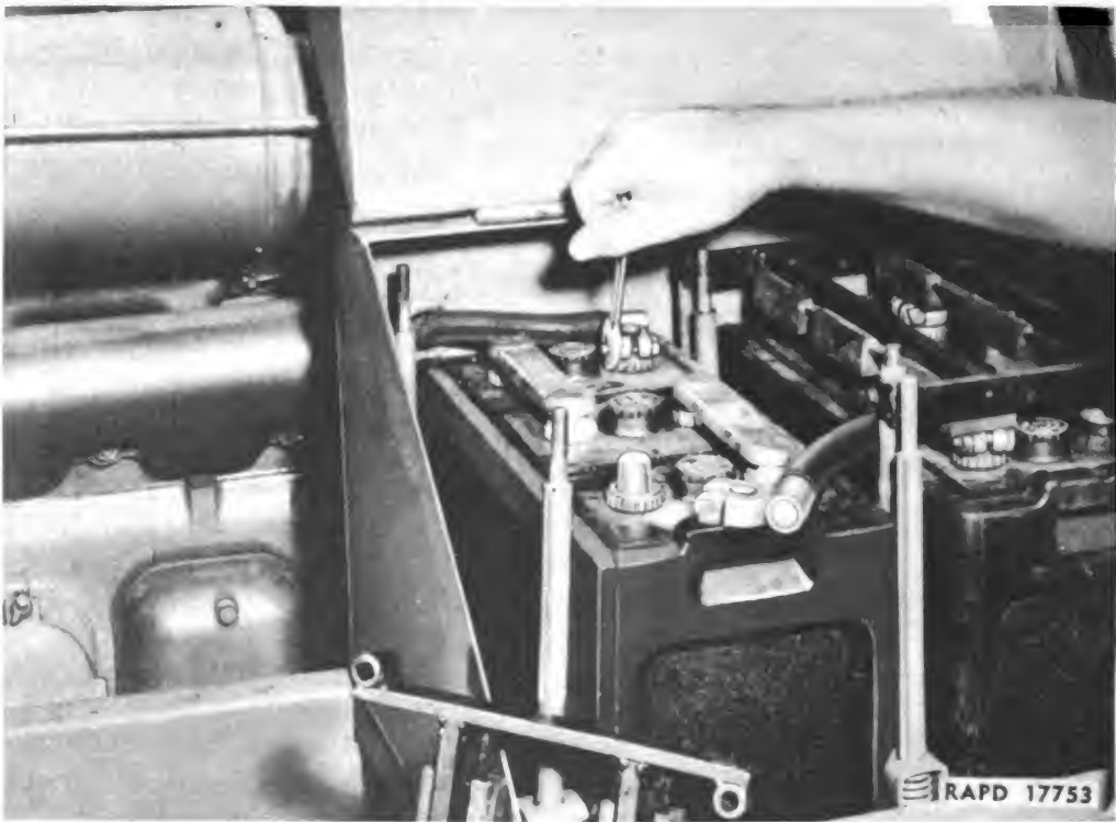
Figure 100—Removing Battery Cable
