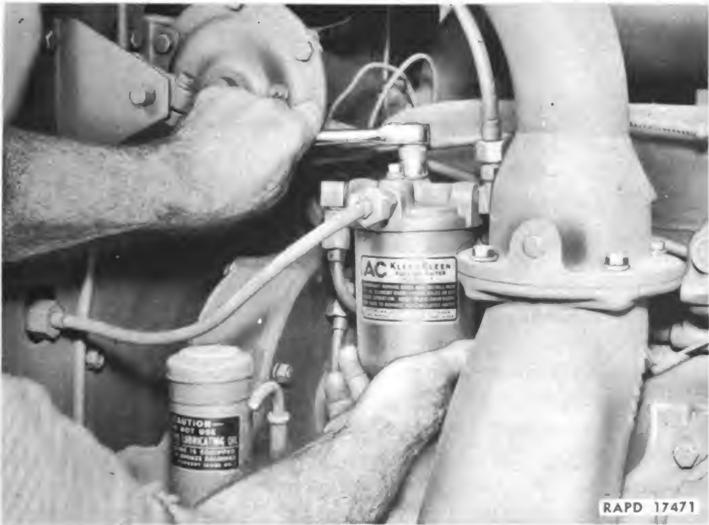
Figure 64—Removing Third Stage Fuel Filter Case
