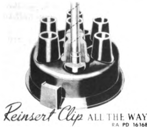
Figure 115—Installing Spark Plug Cables—Distributor Cap
