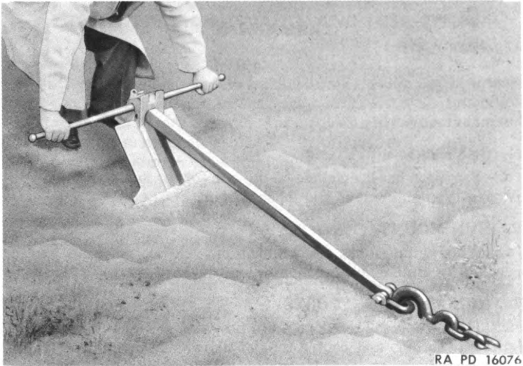
Figure 40—Use of Sand Anchor, May be used in Manner Shown in Figures 22 and 25
