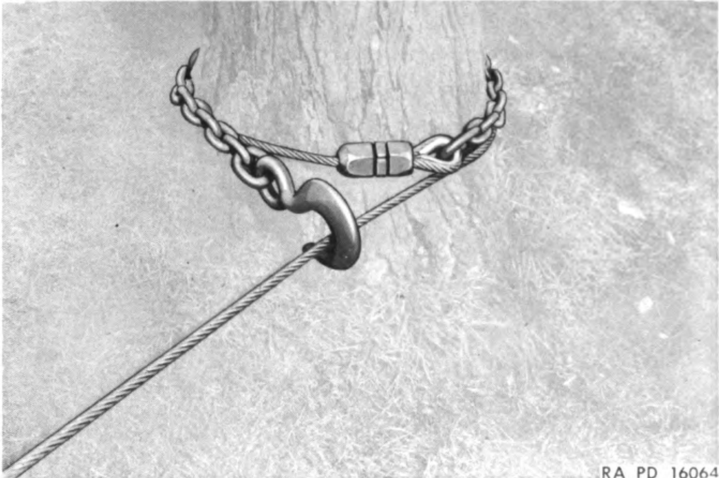
Figure 28—Emergency Hitch Around Tree with Cable as used in Figures 22 and 25
