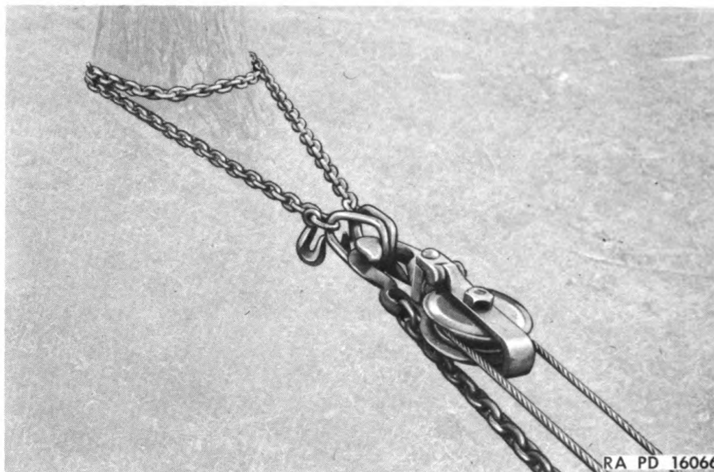
Figure 30—Rigging at Tree with Snatch Block and Chain as used in Figures 20, 23 and 27
