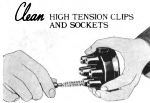
Figure 111—Cleaning Distributor Cap Socket
