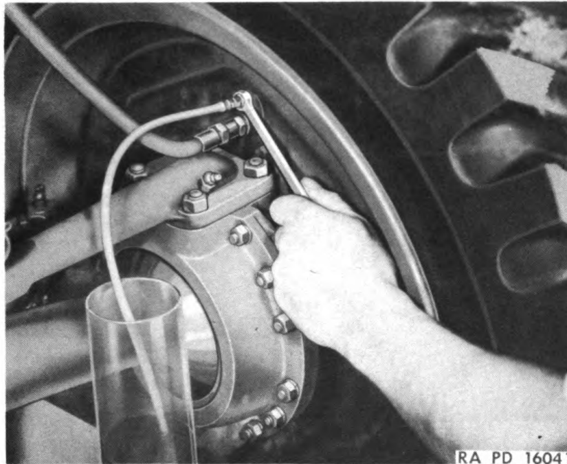
Figure 58—Typical Method of Bleeding Wheel Cylinders
