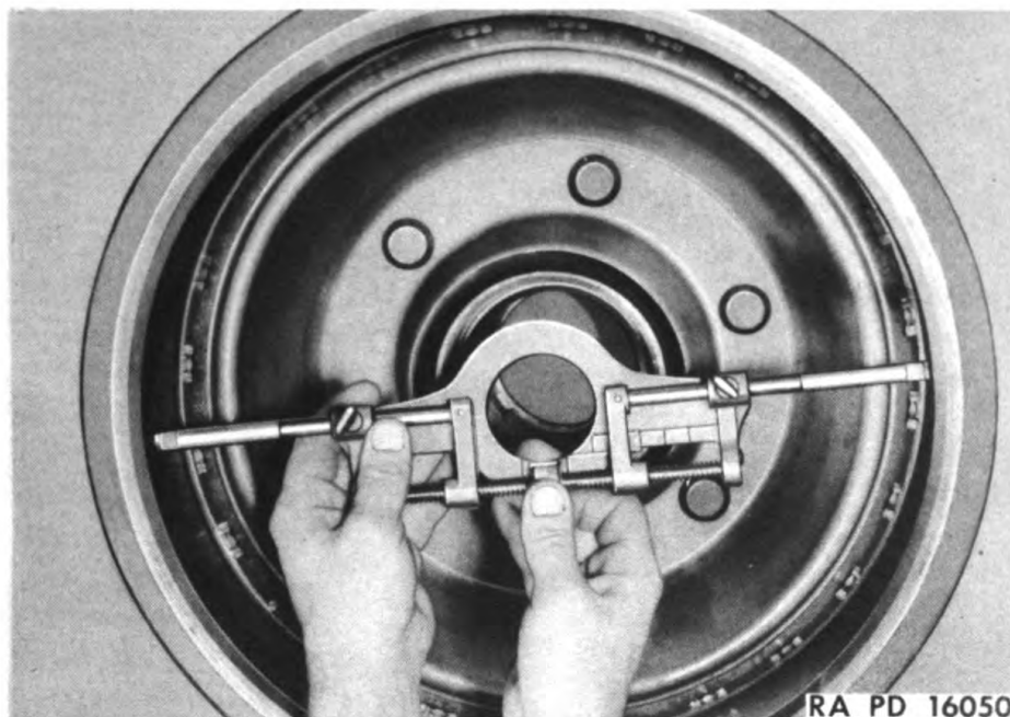
Figure 66—Use of Micrometer to Measure Brake Drum Diameter When Using Lining Grinder
