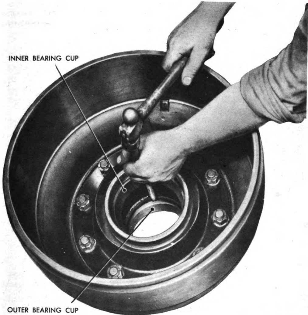
Figure 57—Removing Bearing Cups
